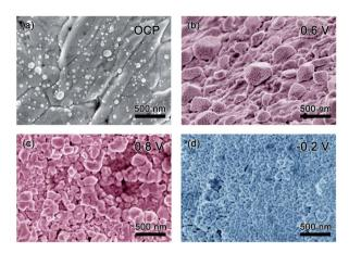
Fig. 4 SEM images of the pristine Ag sample before CV cycling (a) and along CV cycling when the sweep potential stopped at different position: anodic sweep (b) 0.6 V and (c) 0.8 V, cathodic sweep (d) -0.2 V.
