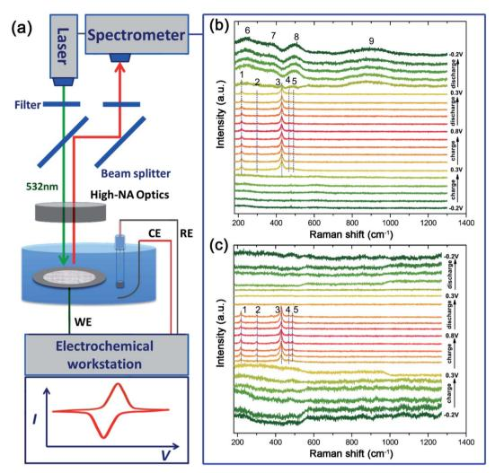
Fig. 6 (a) Schematic of the equipment for *operando* Raman spectroscopy and the *operando* Raman spectra of the pristine silver electrode (b) and the T-Ag electrode (c) collected every 160 seconds during a CV cycle at a sweep rate of 0.625 mV s<sup>-1</sup>.
