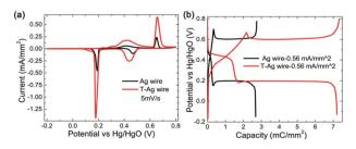
Fig. 3 (a) CV and (b) GCD curves of pristine Ag and the T-Ag and at a same sweep rate and a same charge/discharge current density, respectively.
