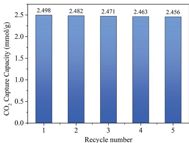
Fig. 10 CO<sub>2</sub> adsorption/desorption cycles for NOMC-L-0.5 at 25 °C.
