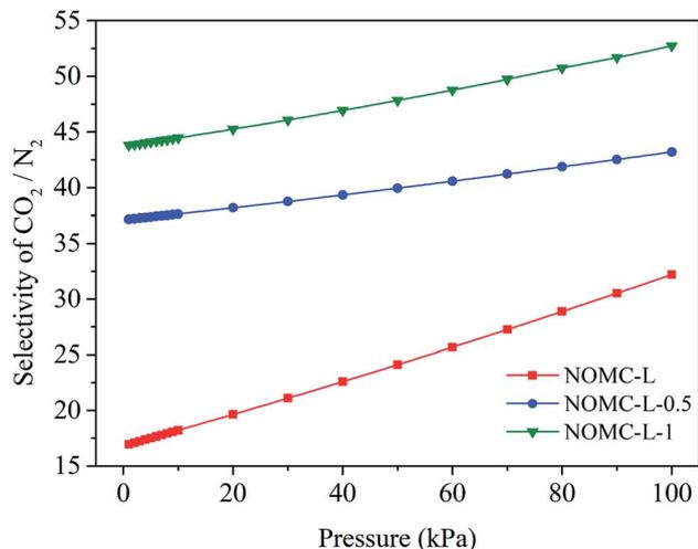
Fig. 9 IAST-predicted selectivity for CO<sub>2</sub>/N<sub>2</sub> (15 : 85) binary mixtures on NOMCs at 25 °C.
