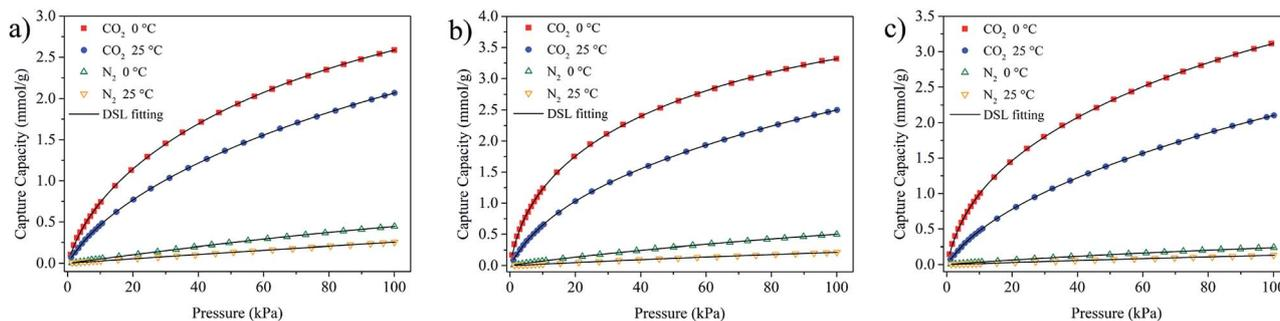
Fig. 7 CO<sub>2</sub> and N<sub>2</sub> adsorption isotherms of NOMC-L (a), NOMC-L-0.5 (b), and NOMC-L-1 (c) (points, experimental data; curves, DSL fitting model) at 0 °C and 25 °C.
