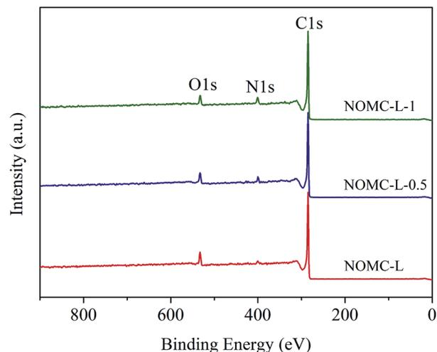
Fig. 5 XPS survey scan spectra of NOMCs.
