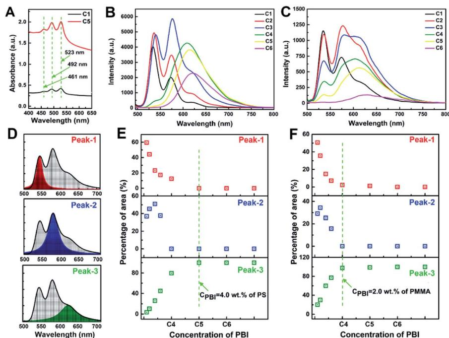
Fig. 3 (A) Absorption spectra of hexylheptyl-PBI/PS with the concentration of C1 and C5. Fluorescence emission spectra of different dye concentrations of hexylheptyl-PBI in PS (B) and PMMA (C) films, respectively. (D) Spectral area of 535 nm (Peak-1, red area), 574 nm (Peak-2, blue area) and 621 nm (Peak-3, green area). Contribution of Peak-1, Peak-2, and Peak-3 to total peak area, versus concentration of hexylheptyl-PBI in PS (E) and PMMA thin films (F).
