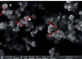
Fig. 2 Scanning electron microscopic images of PLGA- (A) and PEG-PLGA-IFN- $\beta$ -1a (B) nanoparticles.
