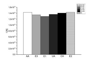
Fig. 11 Effect of interfering substances (50  $\mu$ M) on the determination of E2 level.
