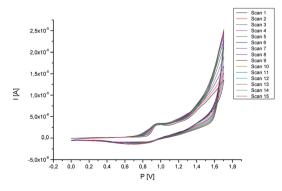
Fig. 4 Stability of the polymer (potential range: 0-1.6 V, scan rate 50 mV s<sup>-1</sup>, number of scans: 10, supporting electrolyte: TBA-TFP solution in dichloromethane).
