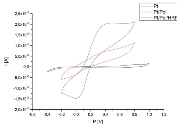
Fig. 7 Representative CV-scans of the bare Pt electrode, Pt electrode modified with polymer and Pt/Pol/HRP system in the presence of 17 $\beta$ -estradiol 10 ( $\mu\text{M}$ ) under applied potential range (potential range  $-0.4$  to  $1.0$  V, scan rate  $100$   $\text{mV s}^{-1}$ , via  $\text{Ag}/\text{AgCl}$ ).
