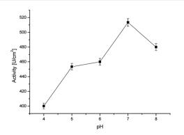
**Fig. 6** Activity of the immobilized horseradish peroxidase at various pH values (at room temperature).
