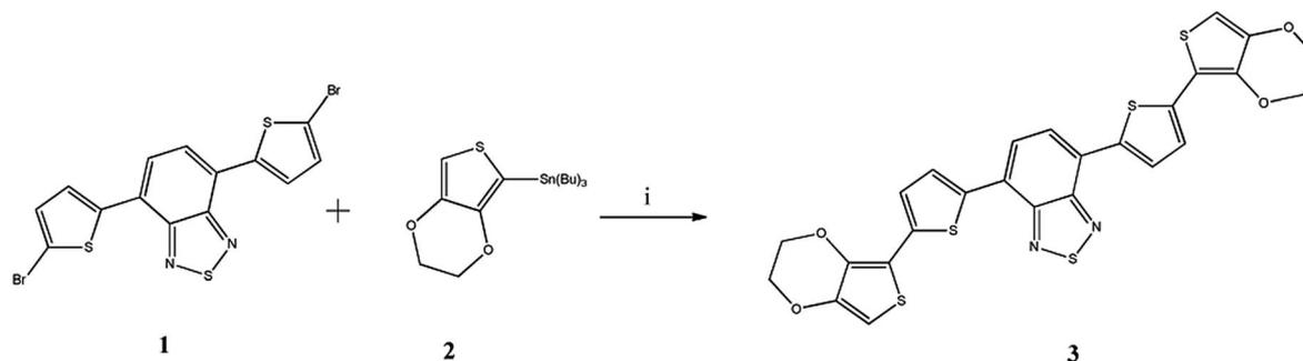
Scheme 1 The synthetic route of the 4,7-bis(5-(3,4-ethylenedioxythiophene)thiophen-2-yl)benzothiadiazole (3). (i) Pd(PPh<sub>3</sub>)<sub>2</sub>Cl<sub>2</sub>, THF, N<sub>2</sub>, 48 h.
