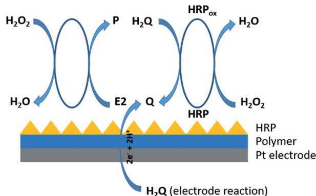
Fig. 2 Schematic representation of the 17 $\beta$ -estradiol enzyme-based biosensor.
