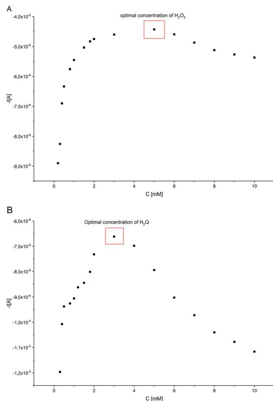
Fig. 8 Variation of the  $I_{p,n}$  for 100  $\mu\text{M}$  of E2 solution in constructed system as a function of: (A)  $C^*\text{H}_2\text{O}_2$  ( $C^*\text{H}_2\text{Q} = 1.0 \times 10^{-3}$  M,  $C^*\text{HRP} = 1.5 \times 10^{-10}$  M); (B)  $C^*\text{H}_2\text{Q}$  ( $C^*\text{H}_2\text{O}_2 = 1.0 \times 10^{-3}$  M,  $C^*\text{HRP} = 1.5 \times 10^{-10}$  M).
