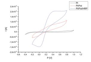
Fig. 7 Representative CV-scans of the bare Pt electrode, Pt electrode modified with polymer and Pt/Pol/HRP system in the presence of 17β-estradiol  $10(\mu M)$  under applied potential range (potential range -0.4 to 1.0 V, scan rate 100 mV s<sup>-1</sup>, via Ag/AgCl).
