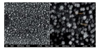
Fig. 5 SEM images for poly[4,7-bis(5-(3,4-ethylenedioxythiophene) thiophen-2-yl)benzothiadiazole] 10  $\mu$ m (A) and 5  $\mu$ m (B).
