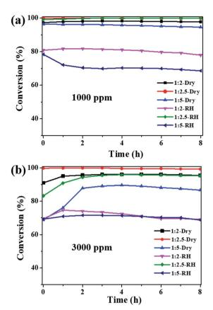
Fig. 4 The conversion of ozone on obtained Cu<sub>2</sub>O catalysts: (a) ozone inlet concentration of 1000 ppm; (b) ozone inlet concentration of 3000 ppm ( $T=25\,^{\circ}$ C, SV = 240 000 mL g $^{-1}$  h $^{-1}$ , dry air or RH  $\sim 90\%$ ).
