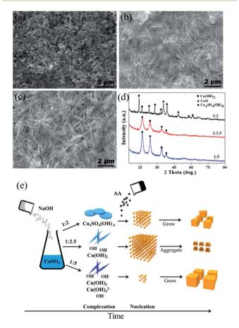
Fig. 3 (a–c) SEM images of precursors obtained at different molar ratios of CuSO<sub>4</sub> and NaOH as 1:2, 1:2.5 and 1:5; (d) XRD of precursors obtained at different molar ratios of CuSO<sub>4</sub> and NaOH as 1:2, 1:2.5 and 1:5; (e) schematic of Cu<sub>2</sub>O formation process under different molar ratios of CuSO<sub>4</sub> and NaOH.
