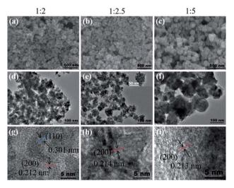
Fig. 2 (a–c) SEM, (d–f) TEM and (g–i) HRTEM images of prepared  $\text{Cu}_2\text{O}$  samples.
