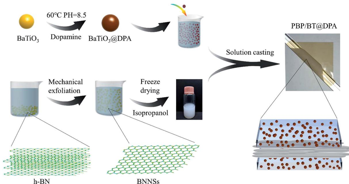
Fig. 1 Experimental flow chart: surface modification of BaTiO<sub>3</sub> by dopamine, preparation of BNNs and fabrication of sandwich structure film.
