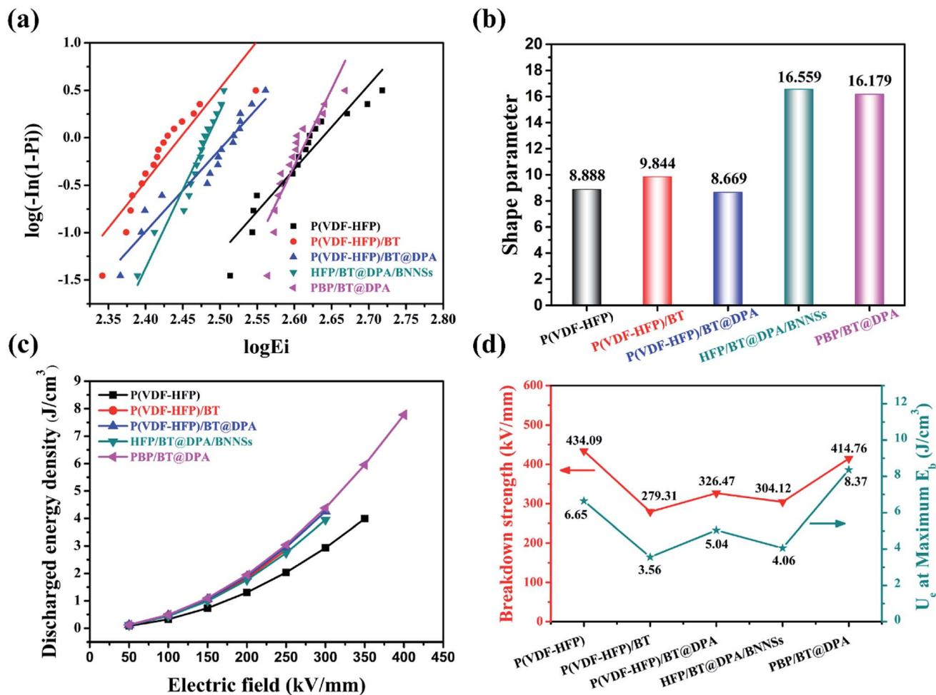
Fig. 5 (a) Weibull distribution, (b) shape factor  $\beta$ , (c) storage density of films under different electric field strengths and (d) the storage density of the films under the maximum breakdown field strength.
