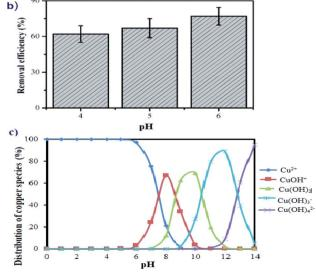
Fig. 4 Adsorption of Cu(II) ions on the manganite surface showing the influence of: (a) the contact time at different pH values; (b) pH of solution at 1 h of contact time and (c) copper species distribution in aqueous solution (modelling with visual MINTEQ 3.1 software, for 25 mg  $\rm L^{-1}$  of copper at 1 atm and 25 °C). The initial copper concentration is 25 mg  $\rm L^{-1}$ .
