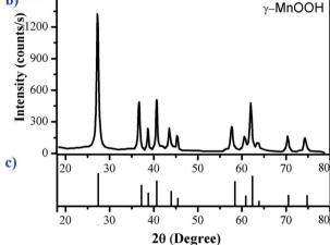
Fig. 1 (a) FTIR-ATR spectrum, (b) X-ray diffraction pattern of manganite sample and (c) diffraction pattern of MnOOH (JCPDS 41-1379).
