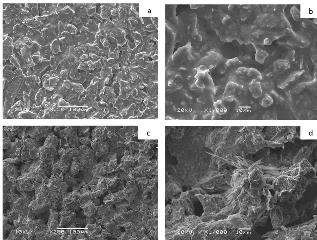
Fig. 5 SEM micrographs: (a and b) low and high magnification images of graphite powder, and (c and d) low and high magnification images of GEG.
