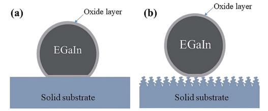
Fig. 2 Wetting state of a LM droplet on different silica glass surfaces: (a) flat silica glass and (b) laser-ablated silica glass
