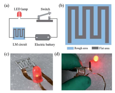
Fig. 5 Preparation of simple LM circuit based on fs laser-induced supermetalphobic microstructures. (a) A circuit composed of LM line, LED lamp, battery, and switch. (b) Construction of the LM circuit. (c and d) Lighting LED lamp up with the as-prepared circuit on different substrates: (c) silica glass and (d) PDMS surfaces.
