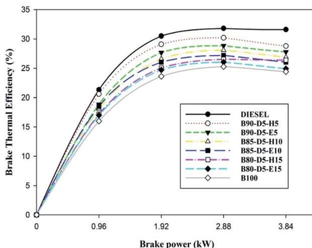
Fig. 6 Variation of BTE with brake power for diesel-biodiesel-alcohol blends.
