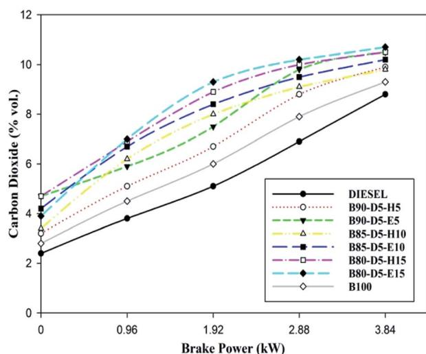
Fig. 10 Variation of CO<sub>2</sub> emission with brake power for diesel-biodiesel-alcohol blends.
