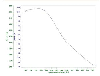
Fig. 4 TGA curve for the Fe<sub>3</sub>O<sub>4</sub>-MWCNTs@PEI-Ag composite.
