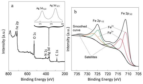
Fig. 5 XPS survey scan for the Fe<sub>3</sub>O<sub>4</sub>-MWCNTs@PEI-Ag composite (a), and high-resolution Ag 3d (inset) and Fe 2p (b) signals.
