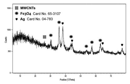
Fig. 2 XRD pattern of the Fe<sub>3</sub>O<sub>4</sub>-MWCNTs@PEI-Ag nanocomposite.
