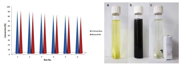
Fig. 9 Left: reusability of the  $Fe_3O_4$ -MWCNTs@PEI-Ag catalyst in reduction of 4-nitroaniline and benzonitrile. Right: photographs of the 4-nitroaniline solution before (a) and after (b) addition of the catalyst, and after magnetic separation of the catalyst (c). The magnet was enveloped with a piece of white paper for clarity.
