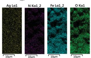
Fig. 6 Mapping analysis of the  $Fe_3O_4$ -MWCNTs@PEI-Ag composite.
