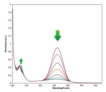
Fig. 8 Trend of reduction for 4-nitroaniline at pH 7.0.
