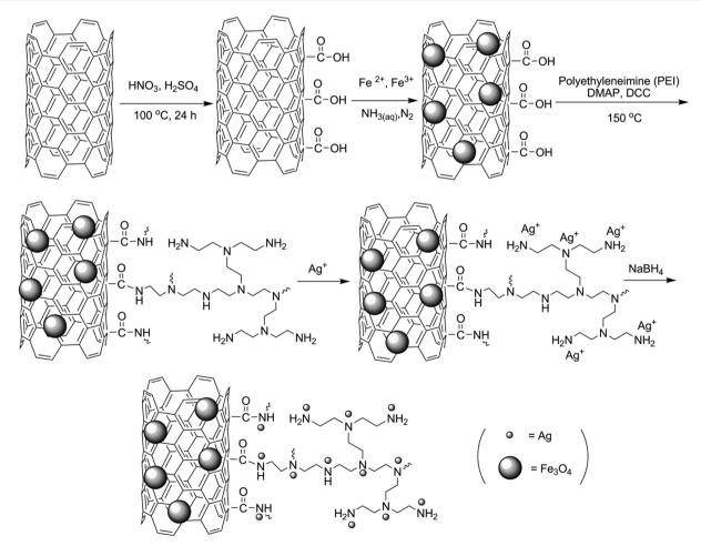
Scheme 1 Stepwise synthesis of Fe<sub>3</sub>O<sub>4</sub>-MWCNTs@PEI-Ag
