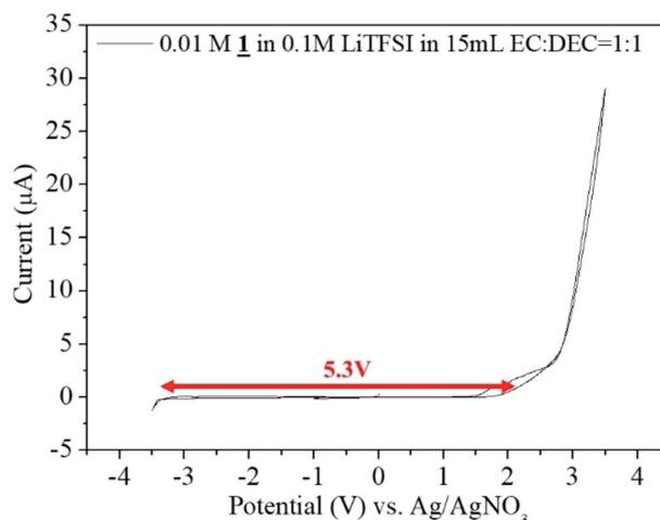
Fig. 7 Cyclic Voltammogram for the sample 1 in 0.1 M LiTFSI in 15 mL EC : DEC = 1 : 1 vs. Ag/AgNO<sub>3</sub>.
