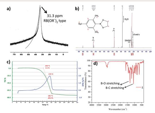
Fig. 2 (a)  $^{11}B$ -NMR of 1 in DMSO- $d_{6x}$  (b)  $^{1}H$ -NMR of 1 in DMSO- $d_{6x}$  (c) TGA profile of 1 (d) IR Spectrum of 1.
