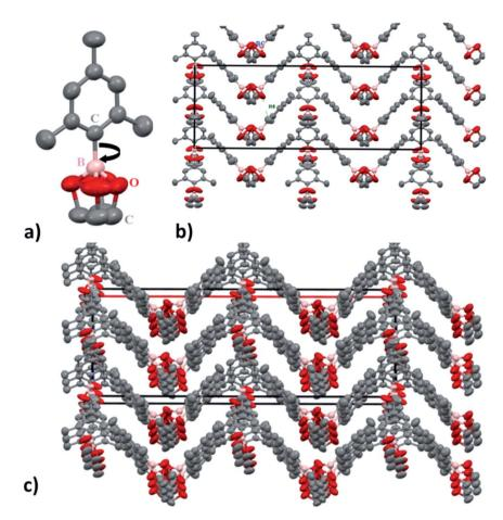
Fig. 5 (a)  $C_9BO_2C_2$  molecule (b) (010) projection of the  $C_9BO_2C_2$  (1) structure. For a better understanding of the real size of the nanochannels (nc), the atoms are represented with their thermal anisotropic ellipsoids. (c) 3D view of the  $C_9BO_2C_2$  (1) structure showing the nanochannels (nc) running along the *b* parameter.
