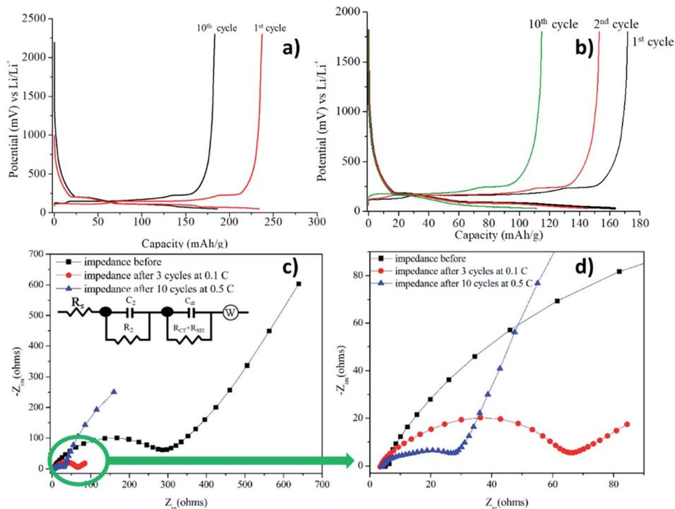
Fig. 8 Charge discharge profiles of 1: LiTFSI = 1 : 2 with 30  $\mu$ L of EC : DEC = 1 : 1 at (a) 0.5C (b) 2C. Inset shows the coulombic efficiency profile of anodic half-cells at corresponding current rates. (c) Impedance analysis before and after charge–discharge with the equivalent circuit, EqC1, used for fitting the charge–discharge data for cell 1, (d) zoom in version of (c).
