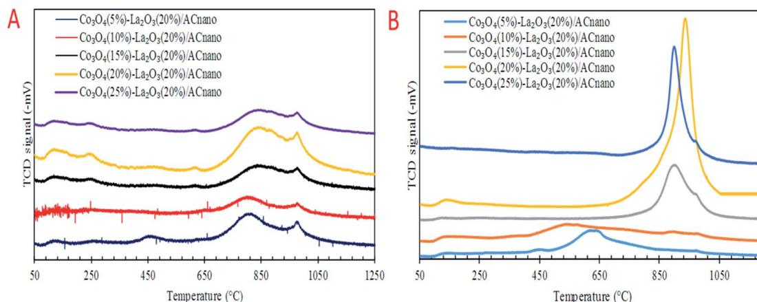
Fig. 3 (A) TPD-NH<sub>3</sub> and (B) TPD-CO<sub>2</sub> profiles for the  $\text{Co}_3\text{O}_4(x)\text{-La}_2\text{O}_3(20)/\text{AC}_{\text{nano}}$  catalysts.
