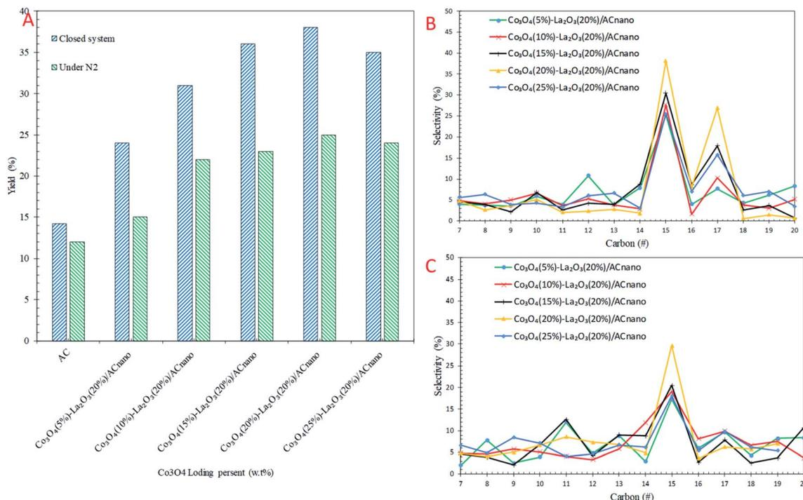
Fig. 4 (A) Effect of Co concentration from 5–25 wt% on (A) hydrocarbon yield, (B) selectivity toward C<sub>8</sub>–C<sub>20</sub> of the micro-batch closed system and (C) selectivity toward C<sub>8</sub>–C<sub>20</sub> under inert conditions with the reaction conditions of 0.5 wt% of catalyst loading, 1 h at 300 °C.
