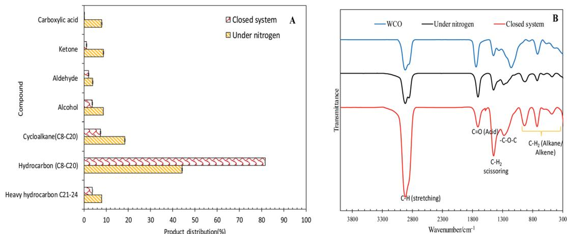
Fig. 5 (A) Product distribution of deoxygenated liquid product analysed by GC-MS and (B) FTIR spectra of the deoxygenized liquid product under the reaction conditions of Co<sub>3</sub>O<sub>4</sub>(20%)-La<sub>2</sub>O<sub>3</sub>(20%)/AC<sub>nano</sub>, 0.5 wt% catalyst loading, 1 h reaction time, and 300 °C reaction temperature.
