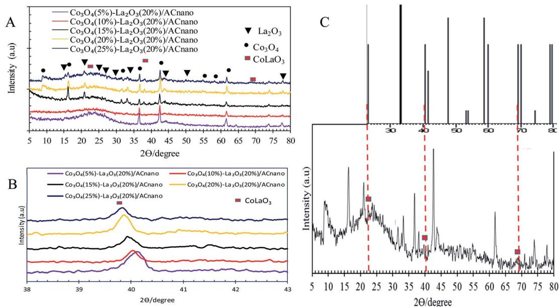
**Fig. 2** (A) XRD patterns of Co<sub>3</sub>O<sub>4</sub>(x)-La<sub>2</sub>O<sub>3</sub>(20%)/AC<sub>nano</sub> catalysts, (B) bimetallic phase shifting and (C) bimetallic phase of CoLa<sub>2</sub>O<sub>3</sub> of Co<sub>3</sub>O<sub>4</sub>(25%)-La<sub>2</sub>O<sub>3</sub>(20%)/AC<sub>nano</sub> catalyst.
