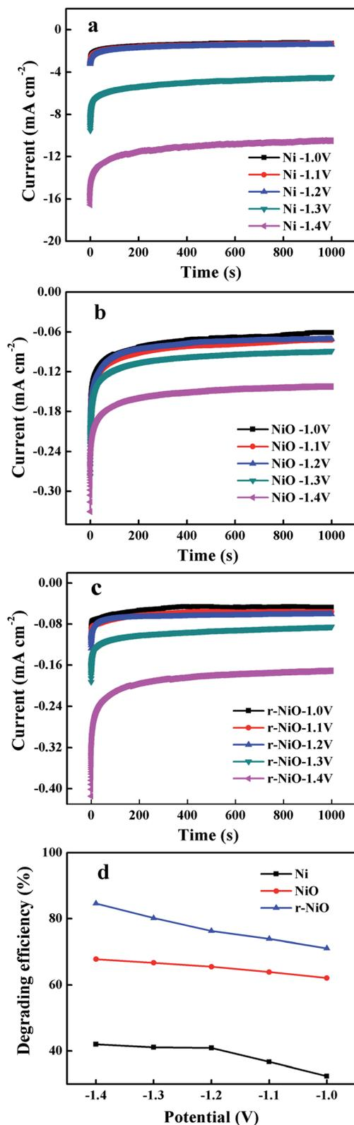
Fig. 6 Current vs. time curves obtained on electrodes of (a) Ni, (b) NiO, (c) r-NiO and (d) degradation efficiency of imidacloprid of the three electrodes at different potentials in 0.1 mol L<sup>-1</sup> NaOH solution.
