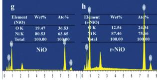
Fig. 2 SEM images of surface view (a–c) and tilted view (d–f) of Ni, NiO and r-NiO, EDS spectra of NiO (g) and r-NiO (h).
