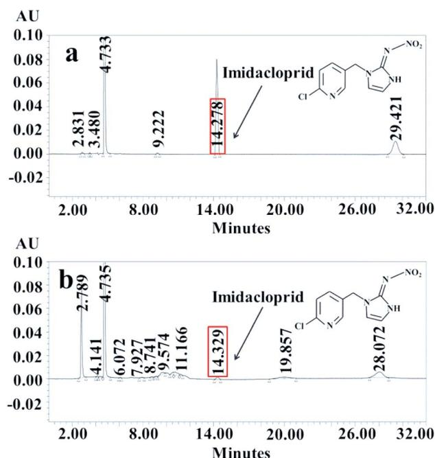
Fig. 7 Analysis results of HLLC-MS before (a) and after (b) electro-reduction of imidacloprid at -1.3 V in 0.1 mol L<sup>-1</sup> NaOH for 1000 s.
