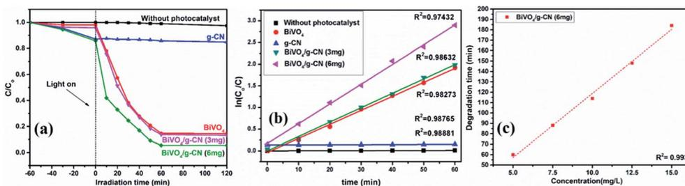
Fig. 5 (a) Photocatalytic degradation of BPB over samples under visible light irradiation. (b) The  $\ln(C_0/C)$  as a function of irradiation time ( $t$ ) for MB degradation. (c) Degradation time of  $\text{BiVO}_4$  and  $\text{BiVO}_4/\text{g-CN}$  (6 mg) as a function of dye concentration ( $5\text{--}15\text{ mg L}^{-1}$ ).
