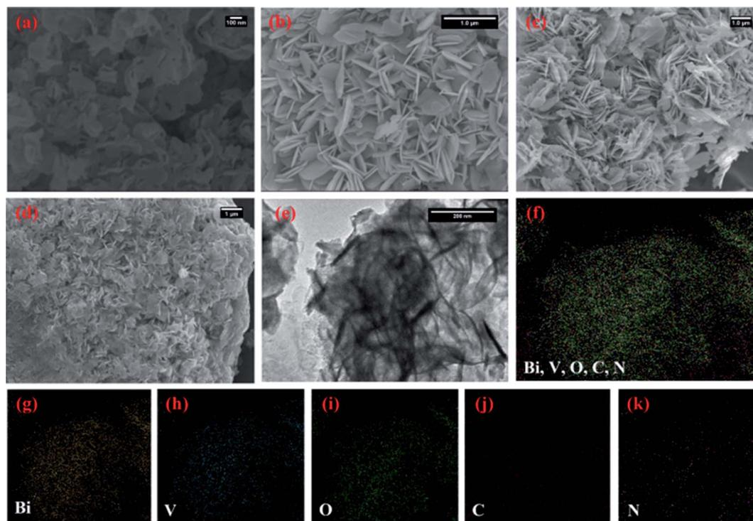
Fig. 2 SEM images of (a) bulk g-CN and (b)  $\text{BiVO}_4$  prepared at  $100^\circ\text{C}$ , (c)  $\text{BiVO}_4/\text{g-CN}$  (3 mg) and (d)  $\text{BiVO}_4/\text{g-CN}$  (6 mg); (e) HRTEM image of  $\text{BiVO}_4/\text{g-CN}$  (6 mg). (f–k) Elemental mapping of  $\text{BiVO}_4/\text{g-CN}$  (6 mg).
