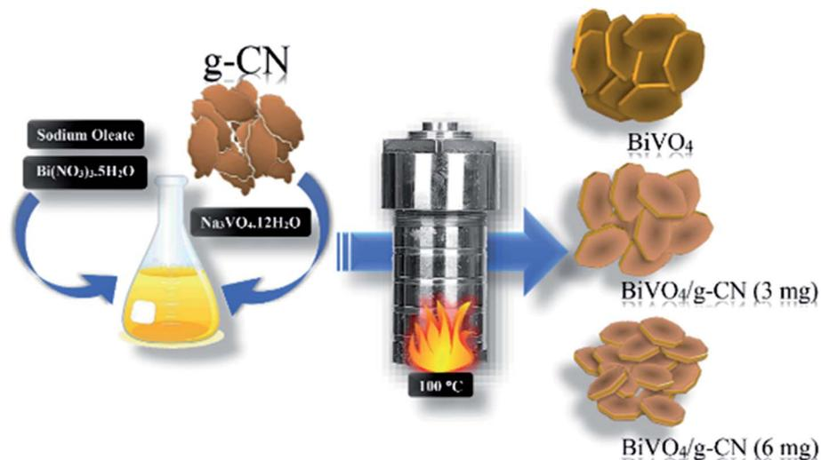
Scheme 1 Schematic illustration of the  $\text{BiVO}_4/\text{g-CN}$  heterostructure photocatalyst system.
