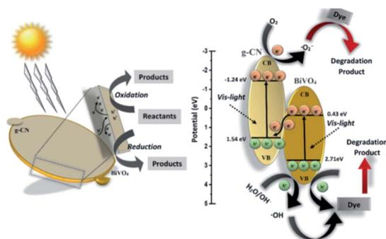
Fig. 11 Schematic illustration of the proposed reaction mechanism in the  $\text{BiVO}_4/\text{g-CN}$  (6 mg) nanocomposite-based reaction system towards dye (MB, BPB) degradation under visible light irradiation.
