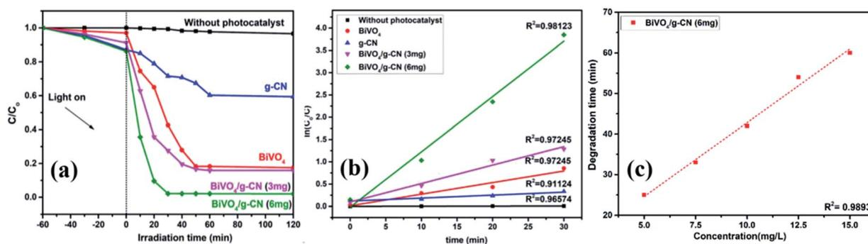
Fig. 4 (a) Photocatalytic degradation of MB over samples under visible light irradiation. (b) The  $\ln(C_0/C)$  as a function of irradiation time ( $t$ ) for MB degradation. (c) Degradation time of  $\text{BiVO}_4$  and  $\text{BiVO}_4/\text{g-CN}$  (6 mg) as a function of dye concentration ( $5\text{--}15\text{ mg L}^{-1}$ ).
