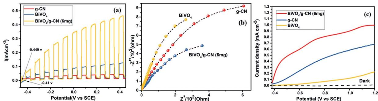
Fig. 8 (a) Transient photocurrent responses of  $\text{BiVO}_4$ , g-CN and  $\text{BiVO}_4/\text{g-CN}$  (6 mg). (b) EIS Nyquist plots of  $\text{BiVO}_4$ , g-CN and  $\text{BiVO}_4/\text{g-CN}$  (6 mg). (c) The cyclic voltammograms of  $\text{BiVO}_4$ , g-CN and  $\text{BiVO}_4/\text{g-CN}$  (6 mg) in dark (dotted curves) and under illumination of simulated AM 1.5G sunlight.
