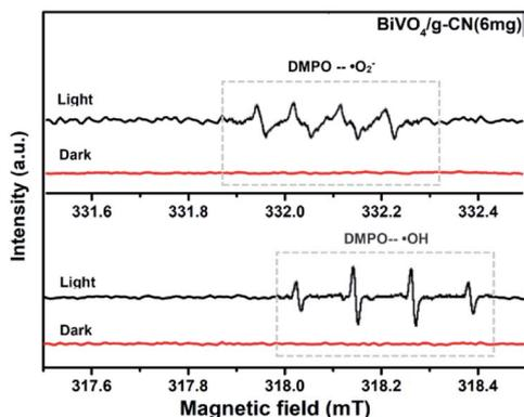
Fig. 10 ESR spectrum of  $\text{BiVO}_4/\text{g-CN}$  samples under irradiation: (a) in methanol dispersion for  $\text{DMPO}-\cdot\text{O}_2^-$  and (b) in aqueous dispersion for  $\text{DMPO}-\cdot\text{OH}$ .
