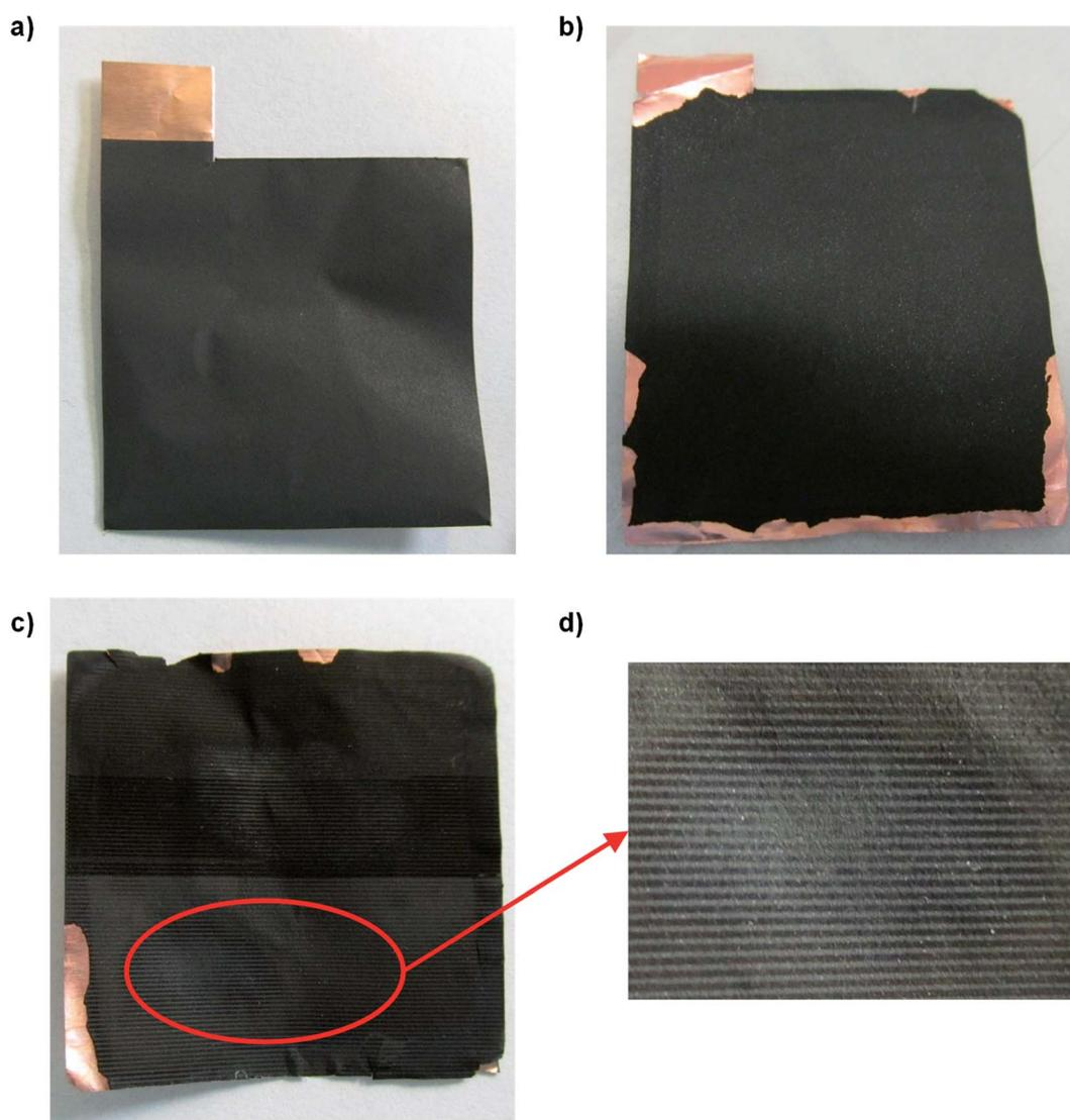
**Fig. 3** Images of the graphitic anodes: (a) pristine anode, (b) cycled anode A, (c) cycled anode B, area of interest (highlighted in red) after the ablation process. (d) Zoomed-in image of the impurity after ablation.
