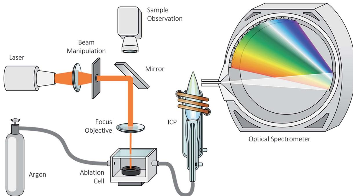
Fig. 1 Schematic set-up of the LA-ICP-OES system.
