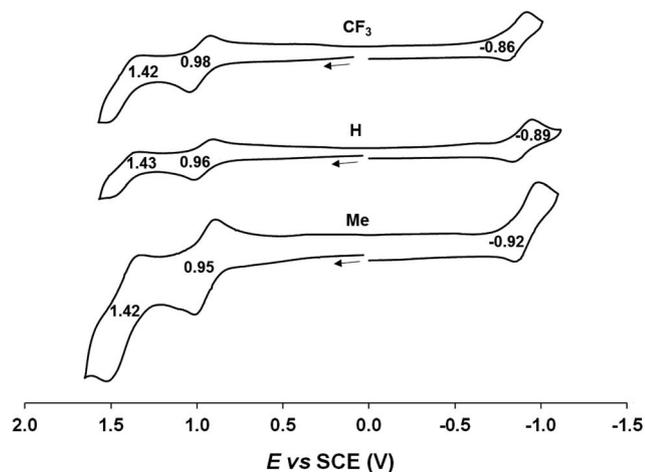
Fig. 5 Cyclic voltammograms of Au[XDPP] (X = CF<sub>3</sub>, H and CH<sub>3</sub>) in benzonitrile. Scan rate: 0.1 V s<sup>-1</sup>.
