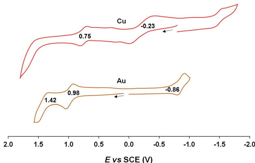
Fig. 6 Cyclic voltammograms of M[CF<sub>3</sub>DPP] (M = Cu and Au) in benzonitrile. Scan rate: for Cu is 0.05 V s<sup>-1</sup> and 0.1 V s<sup>-1</sup> for Au.
