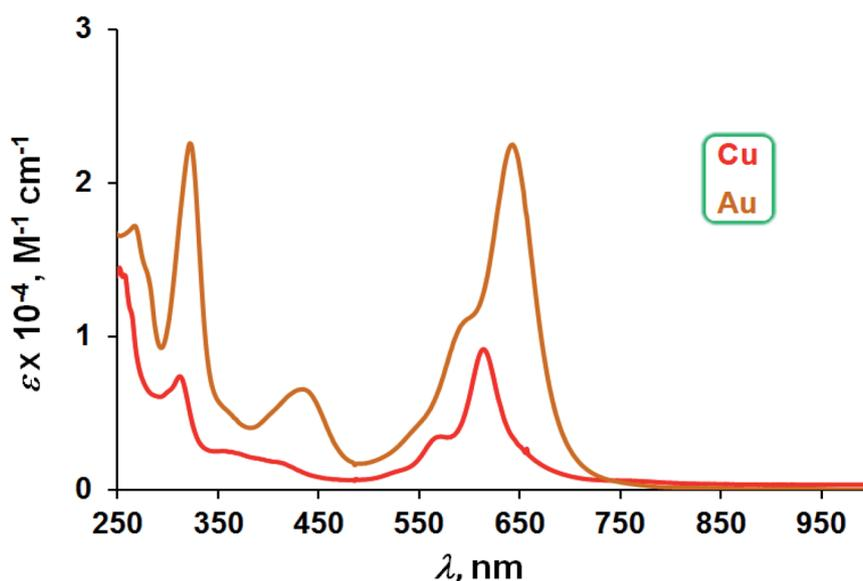
Fig. 4 UV-vis spectra of M[CF<sub>3</sub>DPP] (M = Cu and Au) in dichloromethane.
