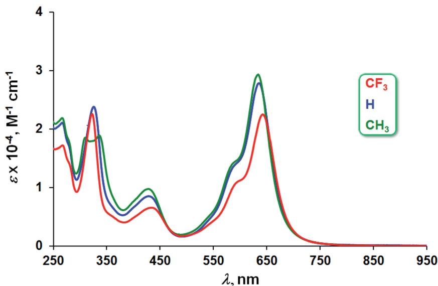
Fig. 3 UV-vis spectra of Au[XDPP] (X = CF<sub>3</sub>, H, and CH<sub>3</sub>) in dichloromethane.
