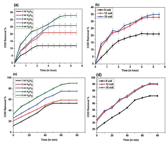
Fig. 2 COD removal % by (a) electrochemical reaction at 12 volts and different concentration of  $H_2O_2$  in mL, (b) electrochemical reactions operated at different applied voltage (9, 12, 15 volts) (c) ZnO NPs formed by different dose of  $H_2O_2$  with power supply of 12 volts, and, (d) ZnO nanoparticles formed at different applied voltage (9, 12, 15 volts).
