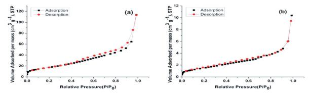
BET-N<sub>2</sub> adsorption-desorption isotherm plots for (a) ZnO nanoparticle (b) ZnO nanoparticle after adsorption of petroleum hydrocarbon (PH).
