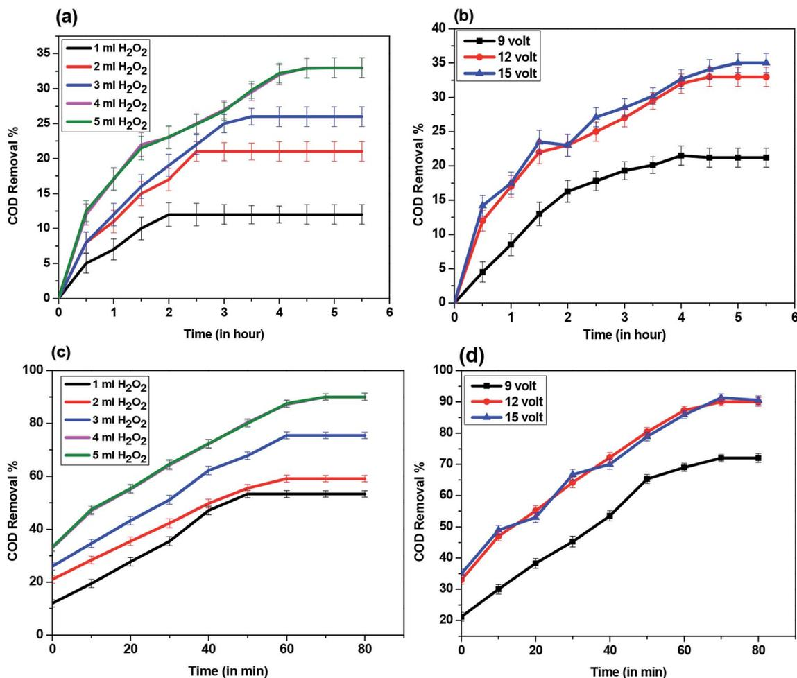
Fig. 2 COD removal % by (a) electrochemical reaction at 12 volts and different concentration of H<sub>2</sub>O<sub>2</sub> in mL, (b) electrochemical reactions operated at different applied voltage (9, 12, 15 volts) (c) ZnO NPs formed by different dose of H<sub>2</sub>O<sub>2</sub> with power supply of 12 volts, and, (d) ZnO nanoparticles formed at different applied voltage (9, 12, 15 volts).
