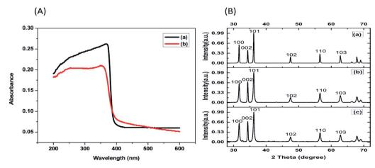
Fig. 3 (A) UV-DRS absorption spectrum of (a) Synthesized ZnO NPs without hydrocarbon, (b) ZnO NPs after adsorption of hydrocarbon. (B) XRD diffraction pattern of (a) commercial ZnO, (b) synthesized ZnO NP without hydrocarbon and (c). Synthesized ZnO after adsorption of hydrocarbon.
