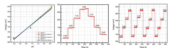
Fig. 6 Sensor response for a group of discrete pH levels from pH 5.45 to pH 8.62. (a) The fitting lines of the three sensors show the linear response with an average sensitivity of 58.57 mV per pH (2.398% RSD). (b) The output response of a pH sensor for increasing and reverse pH buffer solutions. (c) Repetitive results for a group with increasing pH.
