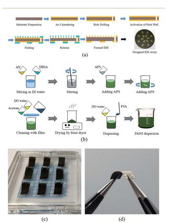
Fig. 4 The fabrication processes of the pH sensor. (a) Process for the PANI membrane preparation. (b) Fabrication process for the interdigital electrodes. (c) Photograph of a group of our fabricated sensors. (d) A sensor bent at approximately 135°.
