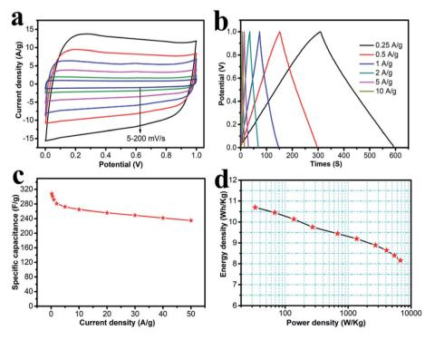
Fig. 6 (a) Cyclic voltammograms of the carbonized CCP/PAA hydrogel composite based on electrode at various scan rates; (b) charge/discharge curves at various current densities; (c) plot of specific capacitance vs. current density; (d) Ragone plot of energy density vs. power density.
