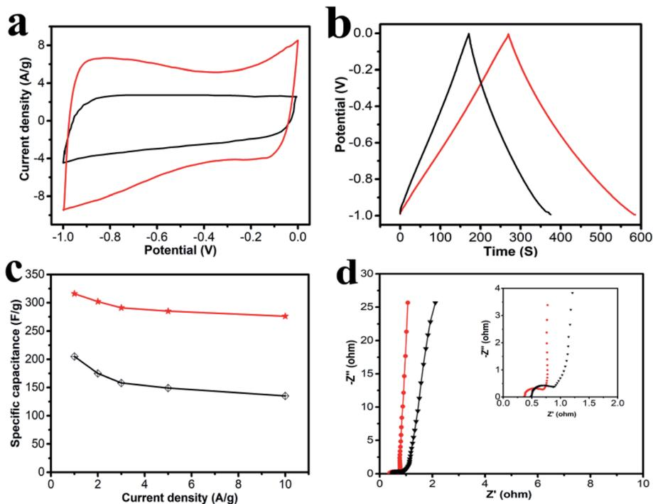
Fig. 5 Electrochemical performances of the carbonized product (black line: HPC-CCP, red line: the HPC-CCP/PAA) measured in a three-electrode system in the 6 M KOH electrolyte: (a) CV curves at  $100 \text{ mV s}^{-1}$ ; (b) galvanostatic charge-discharge curves at a current density of  $1 \text{ A g}^{-1}$ ; (c) specific capacitances at different current densities; (d) the EIS spectra in the frequency range from 10 kHz to 10 mHz (black line: HPC-CCP, red line: the HPC-CCP/PAA).
