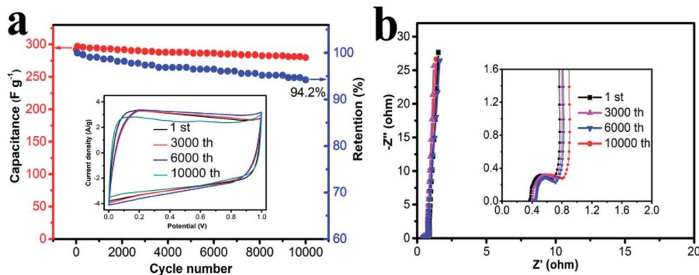
Fig. 7 (a) CV curves of the carbonized CCP/PAA hydrogel composite based electrode at different cycles; (b) Nyquist plots with the inset showing the plots in the high frequency region.
