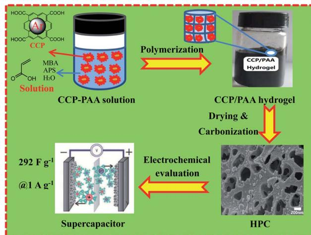
Fig. 1 Schematic representation for the formation of HPC-CCP/PAA.
