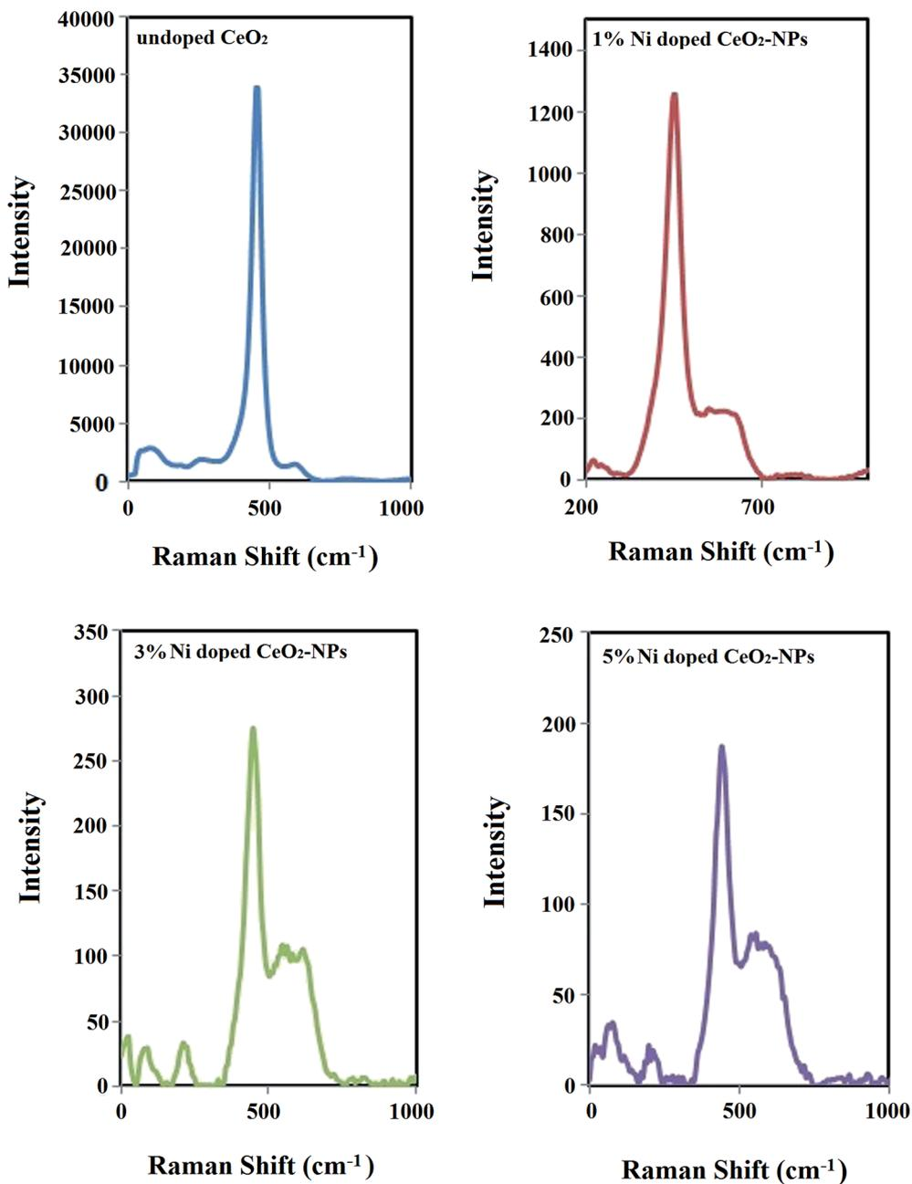
**Fig. 4** Raman spectra of the synthesized undoped and Ni-doped CeO<sub>2</sub>-NPs using the *S. persica* extract.
