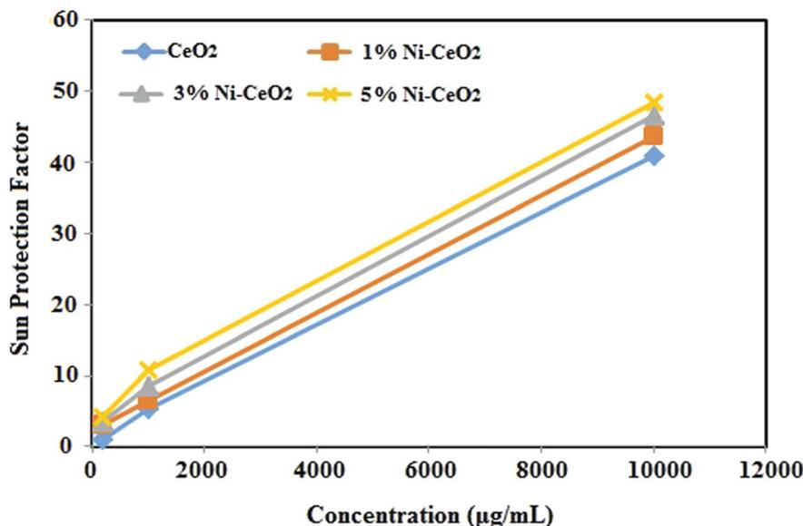
Fig. 10 Sun protection factor (SPF) of the synthesized undoped and Ni-doped CeO<sub>2</sub>-NPs using *S. persica* extract.
