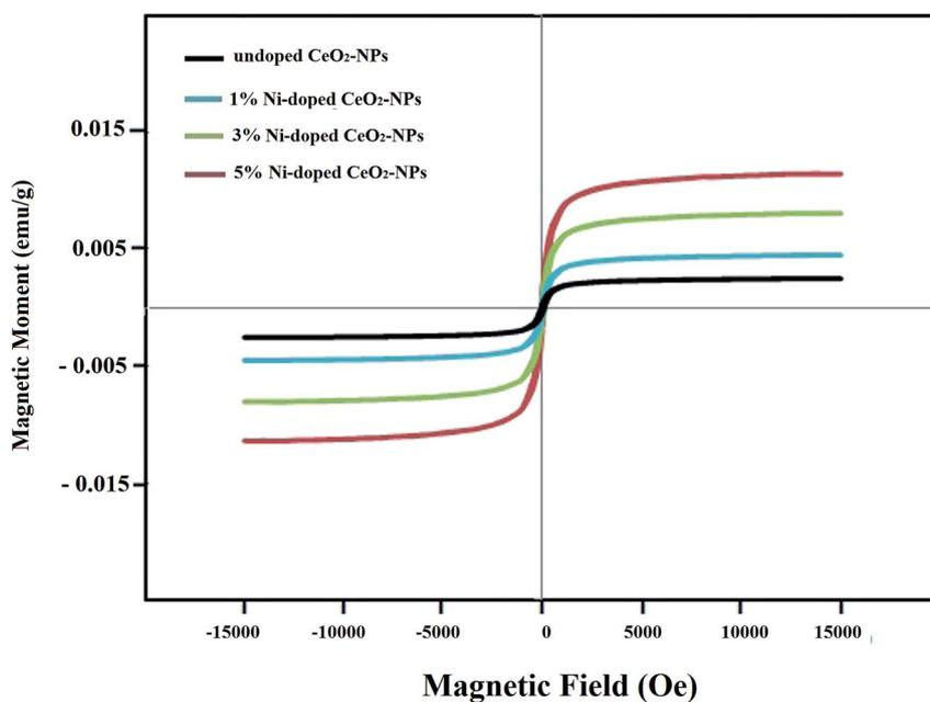
Fig. 7 Magnetic hysteresis curves of the synthesized undoped and Ni-doped CeO<sub>2</sub>-NPs using *S. persica* extract.
