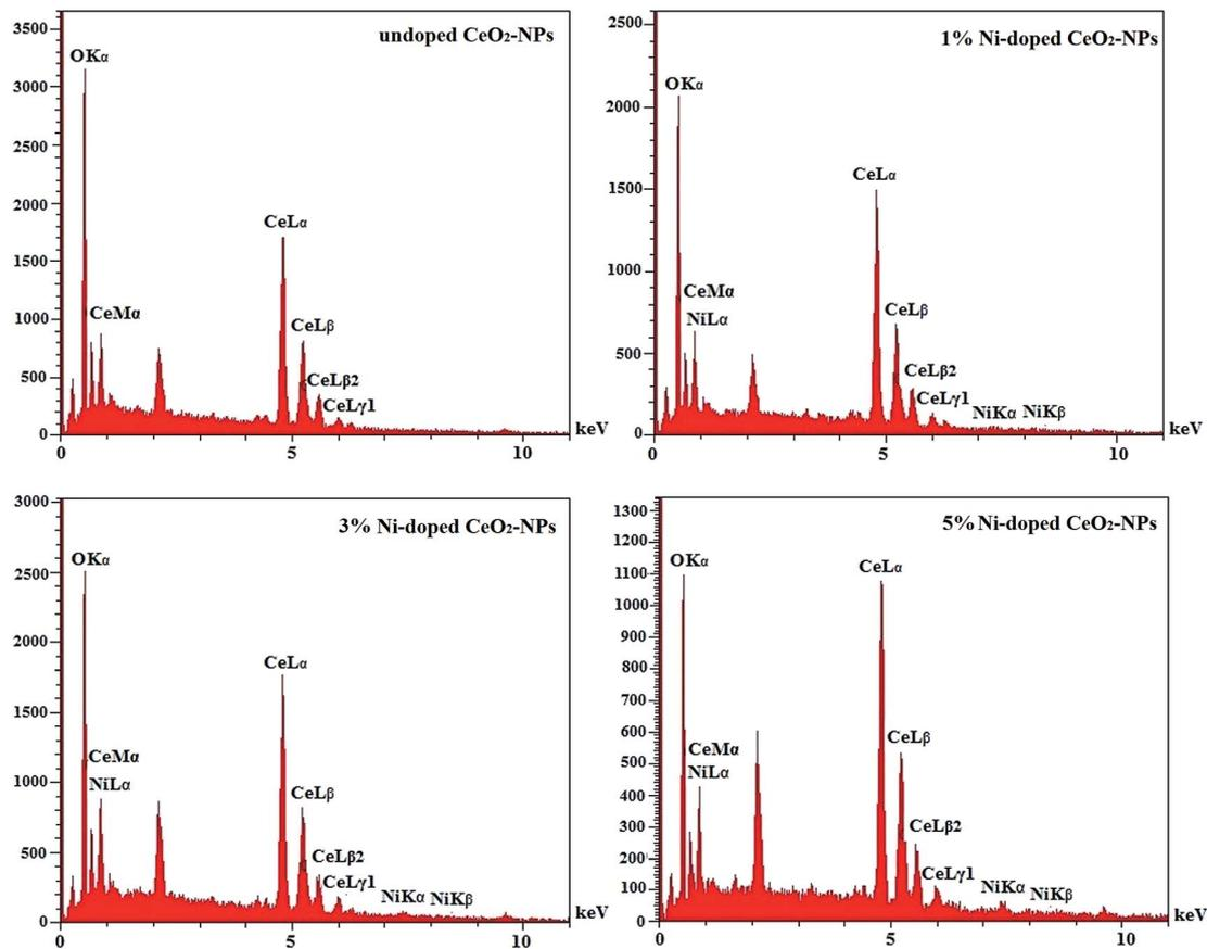
Fig. 6 EDX graph of the synthesized undoped CeO<sub>2</sub>-NPs and Ni-doped CeO<sub>2</sub>-NPs using *S. persica*.
