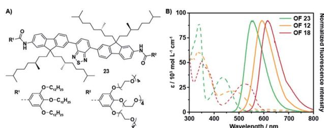
Fig. 2 Comparison of the optical properties between fluorene co-oligomers with and without the bridging vinyl moieties. (A) Molecular structure of OF 23.<sup>38</sup> (B) UV-Vis absorption spectra (dashed lines) and corresponding fluorescence spectra (solid lines) of OFs 12, 18 and 23 in THF ( $c = 1.5 \times 10^{-5}$  M,  $\lambda_{\text{exc}} = 480, 510$  and  $430$  nm, resp.).
