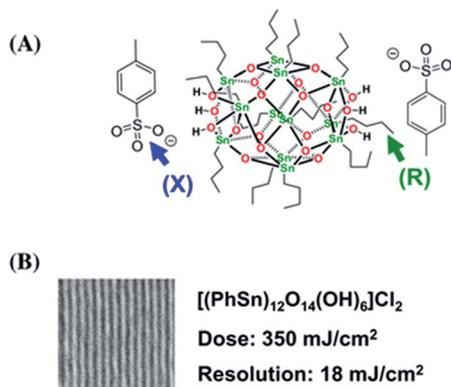
Fig. 10 (A)  $[(\text{BuSn})_{12}\text{O}_{14}(\text{OH})_6]\text{X}_2$  structure, the performance of metal clusters in EUVL was screened by changing anion X and organic ligand R attached to Sn. (B) Lithography results of the best metal cluster obtained by screening, wherein the organic substituent on Sn was benzene, and the anion was chloride ion. Reproduced with permission from ref. 26 Copyright 2014, Elsevier B. V.
