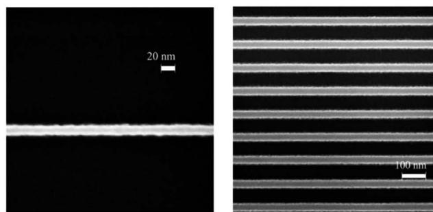
Fig. 6 Left: SEM image of a 15 nm isolate line in ZrCO<sub>2</sub> at a dose of 999  $\mu\text{C cm}^{-2}$ , right: SEM image of 36 nm lines on a 100 nm period in ZrCO<sub>2</sub> at a dose of 810  $\mu\text{C cm}^{-2}$  (30 keV electron-beam). Reproduced with permission from ref. 20 Copyright 2009, Elsevier B. V.
