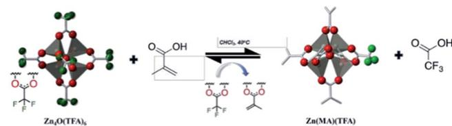
Fig. 15 Synthesis of Zn(MA)(TFA) clusters by using methacrylic acid (MA) to replace trifluoroacetate (TFA) on the surface of Zn<sub>4</sub>O(TFA)<sub>6</sub>. Reproduced with permission from ref. 12. Copyright 2019 SPIE.
