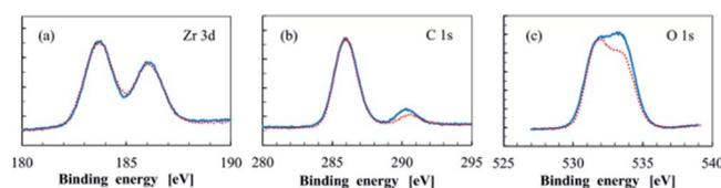
Fig. 7 High resolution XPS spectrum of (a) Zr 3d, (b) C 1s, (c) O 1s in ZrO<sub>x</sub>-MAA metal photoresist, blue represents spectrum before EUV exposure, and red represents XPS after EUV exposure of 20  $\text{mJ cm}^{-2}$ . Reproduced with permission from ref. 22 Copyright 2016 SPIE.
