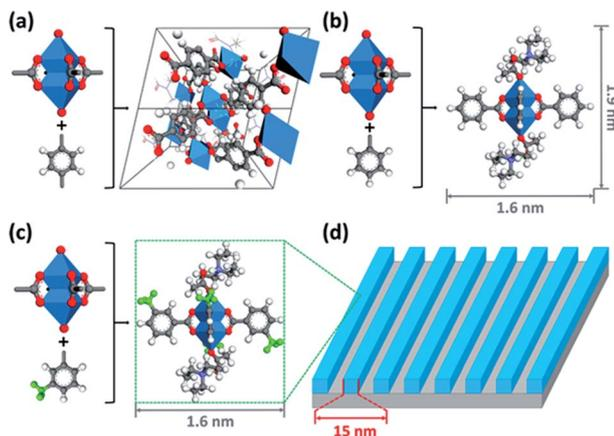
Fig. 14 MOF-2, Zn-BA and Zn-mTA clusters constructed using Zn<sub>2</sub>(CO<sub>2</sub>)<sub>4</sub> containing metal units and organic ligands. (a) Crystal structure of MOF-2. (b) Structure of Zn-BA. (c) Structure of Zn-mTA. (d) A 15 nm HP LS structure could be obtained by photoetching technology using Zn-mTA as photoresist. Atomic color: C – gray. O – red. N – purple. H – white. Zn – blue. Reproduced with permission from ref. 31. Copyright 2015, American Chemical Society.
