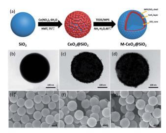
Fig. 1 (a) A schematic drawing of the preparation process of M-CeO<sub>2</sub>@SiO<sub>2</sub>. FESEM and TEM images of the synthesized nanoparticles: (b) SiO<sub>2</sub>-TEM, (c) CeO<sub>2</sub>@SiO<sub>2</sub>-TEM, (d) M-CeO<sub>2</sub>@SiO<sub>2</sub>-TEM, (e) SiO<sub>2</sub>-SEM, (f) CeO<sub>2</sub>@SiO<sub>2</sub>-SEM and (g) M-CeO<sub>2</sub>@SiO<sub>2</sub>-SEM.
