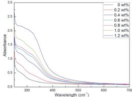
Fig. 6 UV-vis spectra of PF/M-CeO<sub>2</sub>@SiO<sub>2</sub> coatings.
