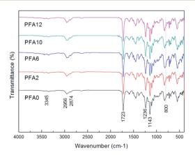
Fig. 5 FT-IR spectra of PF/M-CeO<sub>2</sub>@SiO<sub>2</sub> coatings.
