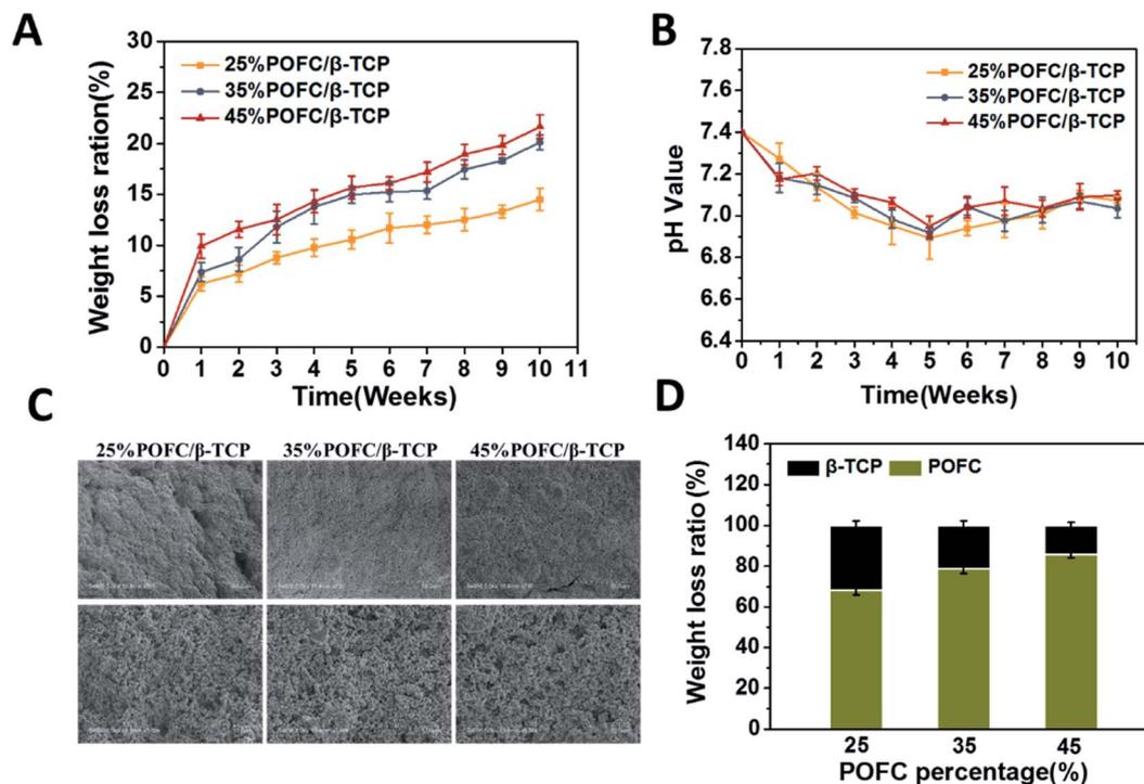
Fig. 5 (A) *In vitro* biodegradation curves of the  $\beta$ -TCP/POFC scaffolds; (B) pH value change of Tris-HCL buffer after immersing the  $\beta$ -TCP/POFC scaffolds; (C) SEM images of composite scaffolds with degradation time of 10 weeks. First row: 700 $\times$ , second row: 5000 $\times$ ; (D) weight loss ratio of  $\beta$ -TCP and POFC in scaffolds at week 10.
