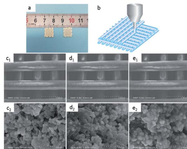
Fig. 3 (a) A photograph of 3D printing POFC/ $\beta$ -TCP scaffold; (b) scaffolds were fabricated via FFS-MDJ printing of the prepared inks; (c–e) SEM images of POFC/ $\beta$ -TCP composite scaffolds at different magnifications; (c1–e1) 40 $\times$ ; (c2–e2) 15 000 $\times$ : (c1 and c2) 25% POFC/ $\beta$ -TCP, (d1 and d2) 35% POFC/ $\beta$ -TCP, (e1 and e2) 45% POFC/ $\beta$ -TCP.
