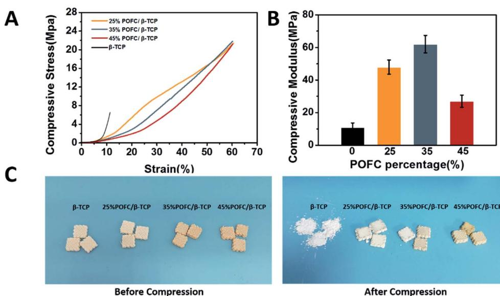
Fig. 4 (A) Typical stress–strain curves of the  $\beta$ -TCP scaffold and  $\beta$ -TCP/POC scaffolds with different POFC contents. (B) Compressive modulus of  $\beta$ -TCP/POC scaffolds with different POFC contents. (C) Photos of scaffolds before and after the compression test. Addition of POFC had improved the mechanical strength, solved the problem of brittleness of  $\beta$ -TCP scaffold.
