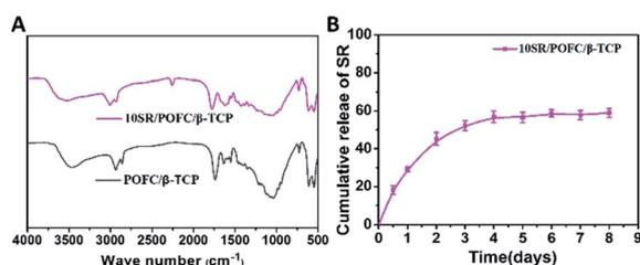
Fig. 7 (A) FTIR of  $\beta$ -TCP/POFC scaffold and SR loaded into  $\beta$ -TCP/POFC scaffold. (B) Cumulative release profiles of SR from  $\beta$ -TCP/POFC scaffold in PBS at  $37\text{ }^{\circ}\text{C}$ .
