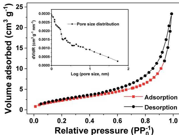
Fig. 2  $N_2$  adsorption-desorption isotherms and corresponding pore size distribution curve (the inset) of the Sn/SnO sample.
