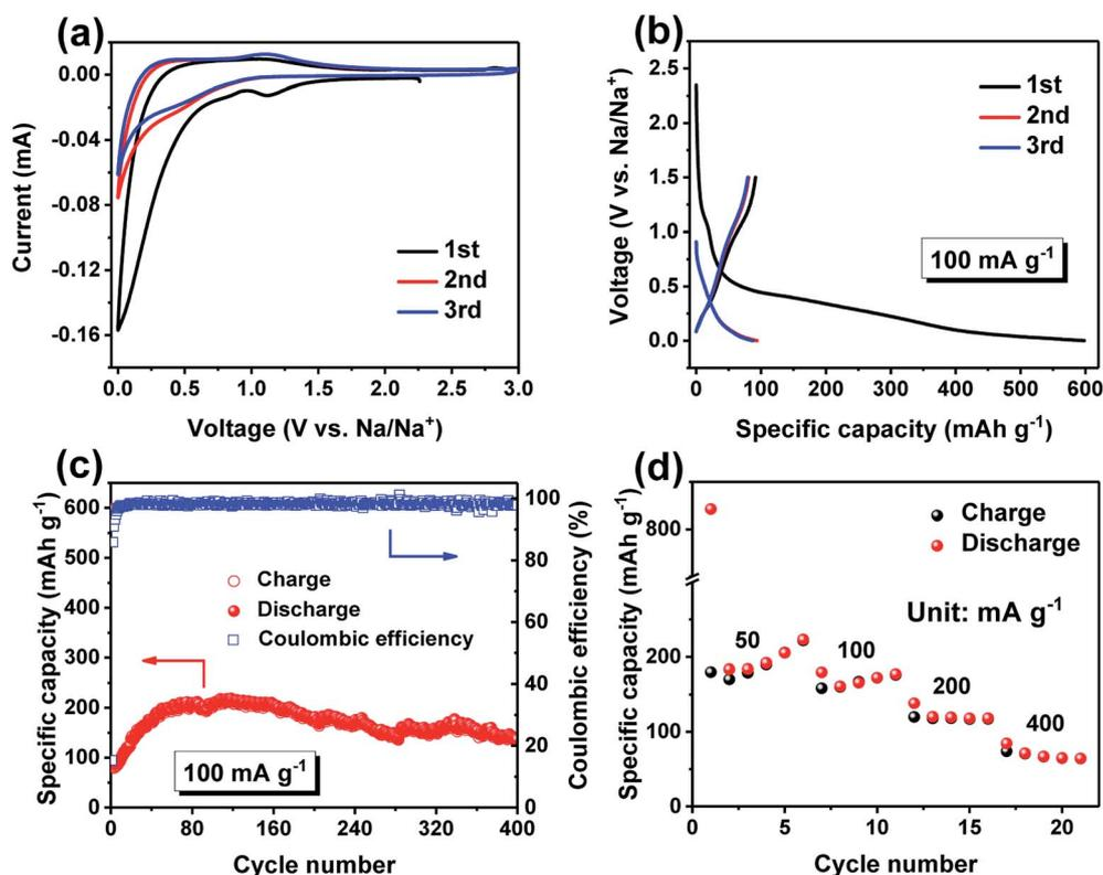
Fig. 6 (a) CV curves of the first three cycles at  $0.1 \text{ mV s}^{-1}$ , (b) galvanostatic charge-discharge curves for the first three cycles at  $100 \text{ mA g}^{-1}$ , (c) cycling performance at  $100 \text{ mA g}^{-1}$ , (d) rate performances of the Sn/SnO sample.
