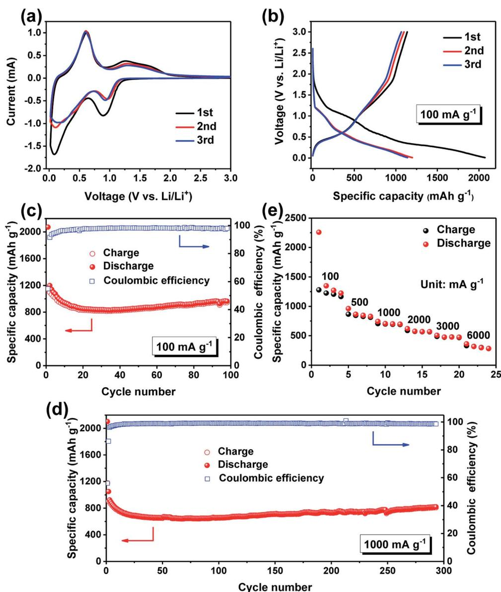
Fig. 4 (a) CV curves of the first three cycles at  $0.1 \text{ mV s}^{-1}$ , (b) galvanostatic charge–discharge curves for the first three cycles at  $100 \text{ mA g}^{-1}$ , (c and d) cycling performances at 100 and  $1000 \text{ mA g}^{-1}$ , (e) rate performances of the Sn/SnO sample.
