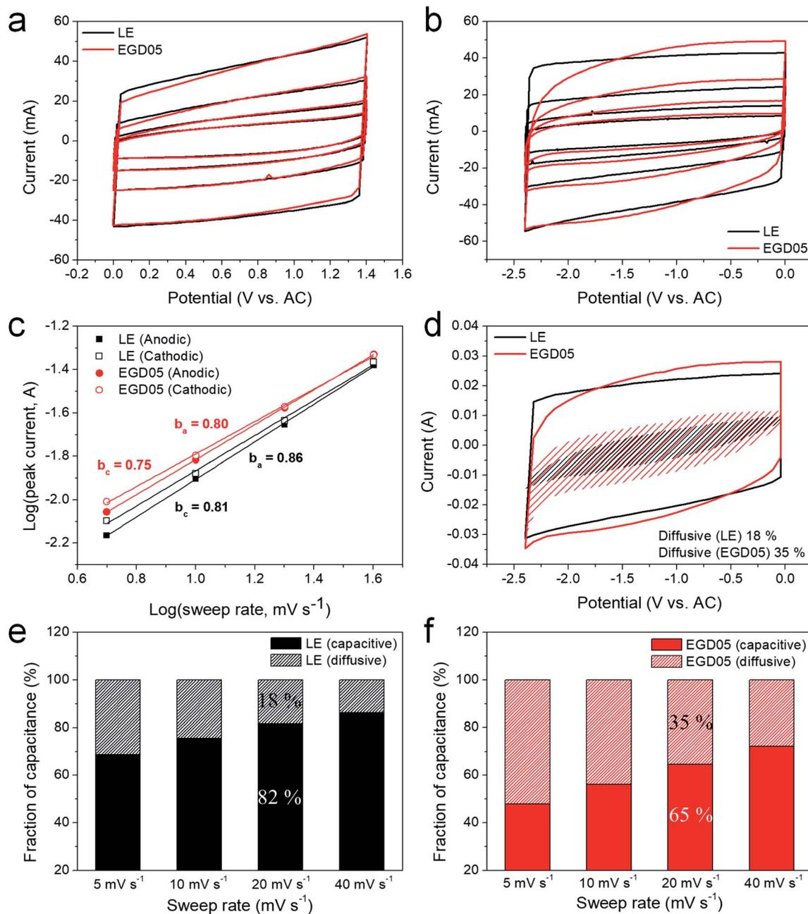
Fig. 1 CVs on (a) positive and (b) negative AC electrodes at 5, 10, 20, 40  $\text{mV s}^{-1}$ . (c) Specific currents at various rates. (d) CV curves representing total (solid line) and diffusive current (shaded region) at 20  $\text{mV s}^{-1}$ . Fraction of capacitance of (e) LE and (f) EGD05 at various rates.
