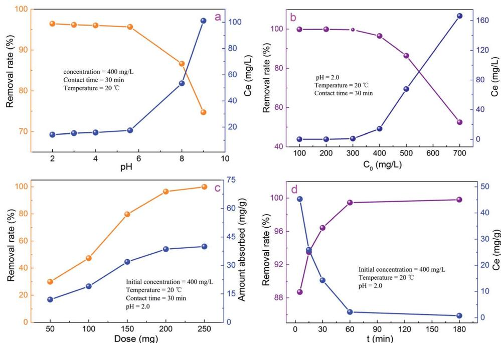
Fig. 3 Effect of pH (a), initial concentration (b), dose (c) and contact time (d) on the Cr(vi) removal of the PPY/Fe<sub>3</sub>O<sub>4</sub>/ATP composite.
