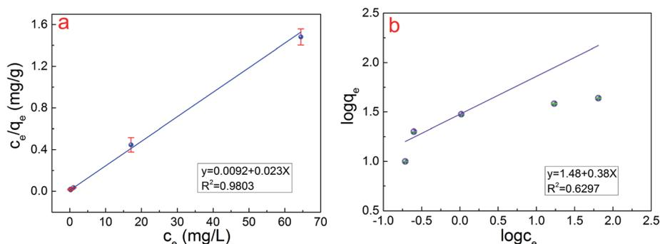
Fig. 6 (a) Langmuir and (b) Freundlich isotherms for Cr(vi) removal by PPy/Fe<sub>3</sub>O<sub>4</sub>/ATP composite.
