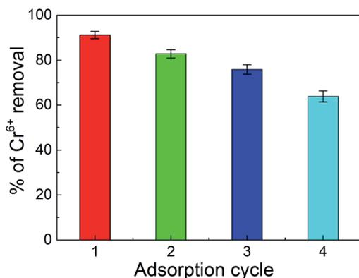
Fig. 7 Desorption and regeneration of PPy/Fe<sub>3</sub>O<sub>4</sub>/ATP composite.
