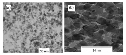
Fig. 5 TEM images of (a) Ag and (b) NiO nanoparticles.
