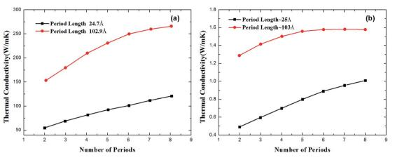
Fig. 3 Thermal conductivities of diamond SLNWs (a) and SiGe SLNWs (b) versus the number of periods
