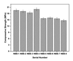
Fig. 7 The compressive strengths of NBB. NBB-1 to 4: bricks made <sup>a</sup> Limits in GB 5085,3-2007, from ES-B. NBB-5 to 8: bricks made from ES-A.
