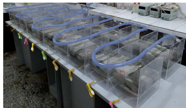
Fig. 2 Experimental rainfall simulation device in operation.
