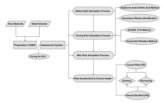
Fig. 4 The main experimental flowchart.
