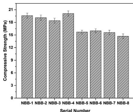
Fig. 7 The compressive strengths of NBB. NBB-1 to 4: bricks made from ES-B, NBB-5 to 8: bricks made from ES-A.
