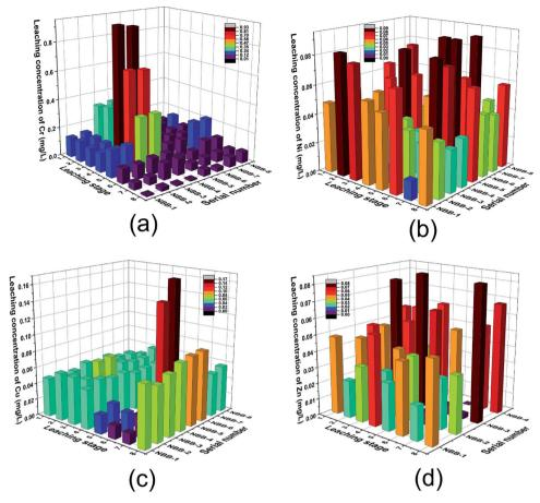
Leaching concentration of HMs at different leaching stages i.e. (a) Cr, (b) Ni, (c) Cu and (d) Zn
