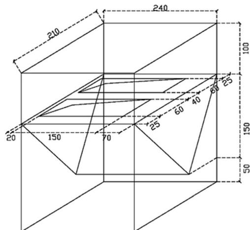
Fig. 1 The design of an experimental rainfall-simulation device.
