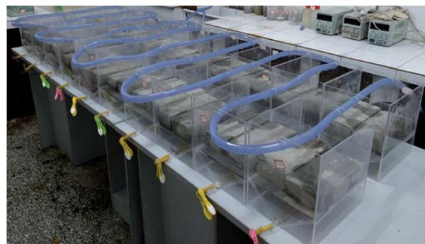
Fig. 2 Experimental rainfall simulation device in operation.
