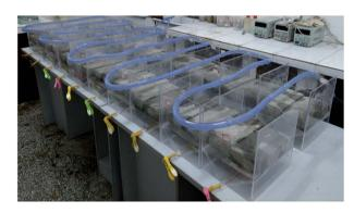
Fig. 2 Experimental rainfall simulation device in operation.
