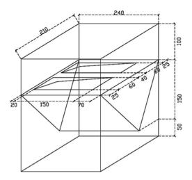
Fig. 1 The design of an experimental rainfall-simulation device
