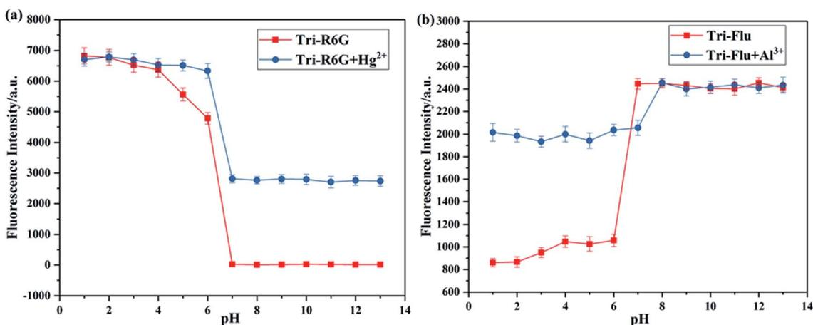
Fig. 7 Fluorescence response of sensor Tri-R6G (a) and Tri-Flu (b) (10  $\mu$ M) as a function of pH (pH 1.0–13.0) in the absence and presence of Hg<sup>2+</sup> and Al<sup>3+</sup> (10  $\mu$ M), respectively, at room temperature.
