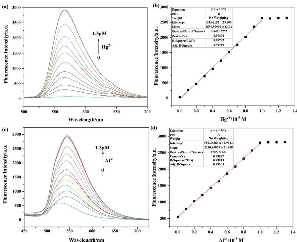
Fig. 4 The fluorescence spectra of Tri-R6G (a) and Tri-Flu (c) ( $10 \mu\text{M}$ ) with the increasing concentration of  $\text{Hg}^{2+}$  and  $\text{Al}^{3+}$  ions ( $0$ – $1.3 \mu\text{M}$ ) in DMSO/ $\text{H}_2\text{O}$  ( $7/3$ , v/v) and ethanol, respectively; the linear fit between Tri-R6G (b) with  $\text{Hg}^{2+}$  ions and Tri-Flu (d) with  $\text{Al}^{3+}$  ions.
