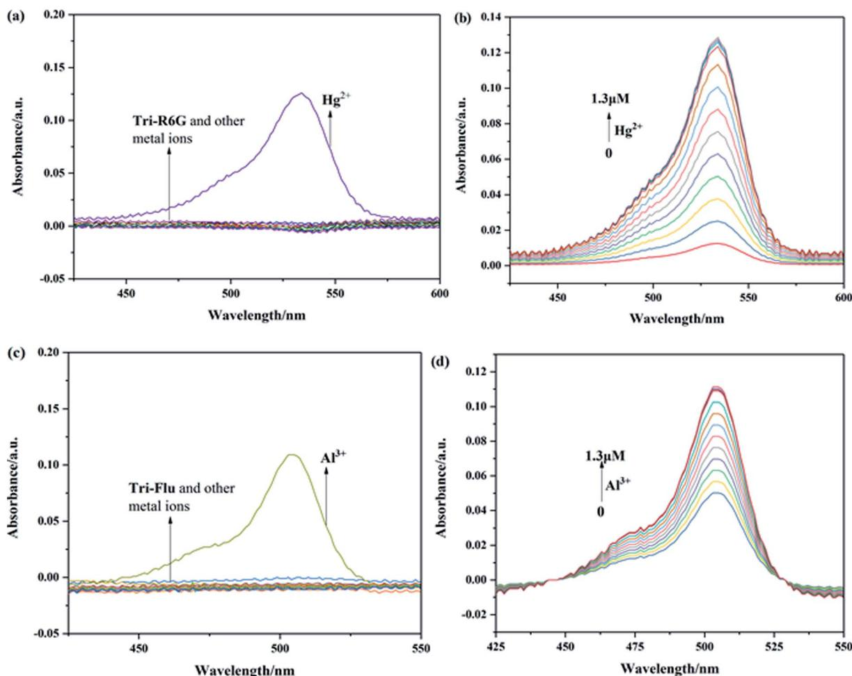
Fig. 1 UV-visible absorption of Tri-R6G (a) and Tri-Flu (c) in the presence and absence of different metal ions in a mixed solution of DMSO/H<sub>2</sub>O (7/3, v/v) at 25 °C. (b) and (d) Upon titration with Hg<sup>2+</sup> and Al<sup>3+</sup> ( $1 \times 10^{-5}$  M, 0–1.3  $\mu\text{M}$ ), respectively.
