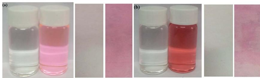
Fig. 10 (a) Photographs showing the color change of the sensor Tri-R6G solution and test strips in a water sample containing no  $\text{Hg}^{2+}$  and water samples in the river. (b) Photographs showing the color change of the sensor Tri-Flu solution and test strips in a water sample containing no  $\text{Al}^{3+}$  and water samples in the river.
