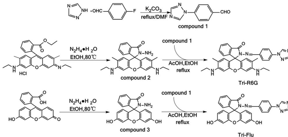
Scheme 1 Synthesis of probes Tri-R6G and Tri-Flu.
