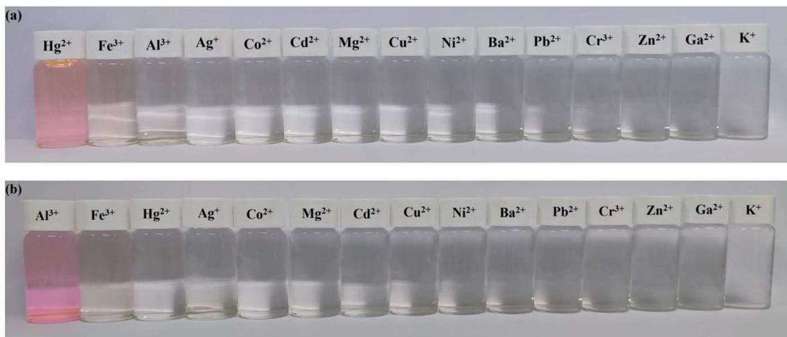
Fig. 8 Colorimetric performance of sensor Tri-Flu +  $\text{Hg}^{2+}$  (a) ( $10\ \mu\text{M}$ ) and Tri-R6G +  $\text{Al}^{3+}$  (b) ( $10\ \mu\text{M}$ ) upon addition of different metal ions ( $1.0\ \mu\text{M}$ ) in DMSO/ $\text{H}_2\text{O}$  (7/3, v/v) solution and ethanol solution.
