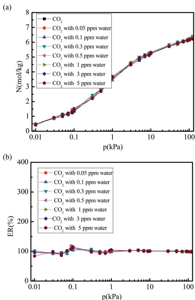
Fig. 6 Simulated  $CO_2$  adsorption equilibrium isotherm and adsorption percent in 5A zeolite under different amounts of trace water vapor without considering the effect of the electrostatic interactions of water molecule. (a)  $CO_2$  adsorption isotherm in 5A zeolite without considering the effect of the electrostatic interaction of molecule. (b) Percent of  $CO_2$  adsorption amount without considering partial charges of water molecule.
