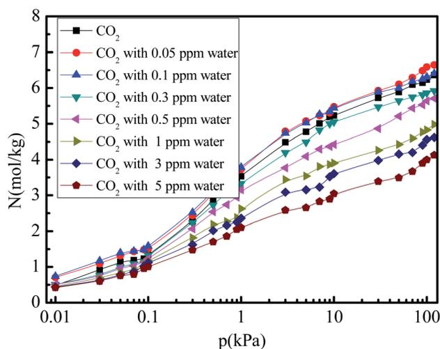
Fig. 3 Simulated CO<sub>2</sub> adsorption equilibrium isotherms in 5A zeolite under different amounts of trace water vapor.
