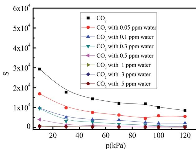
Fig. 8 Simulated CO<sub>2</sub>/(N<sub>2</sub> + O<sub>2</sub>) gas mixture selectivity under different amounts of trace water vapor.
