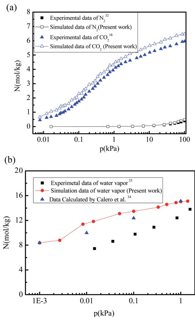
Fig. 2 Comparison of the simulation results with experimental data and with the simulation results reported in the literature. (a) Adsorption isotherms of CO<sub>2</sub> and N<sub>2</sub> adsorbed in 5A zeolite. (b) Adsorption isotherms of water vapor adsorbed in 5A zeolite.
