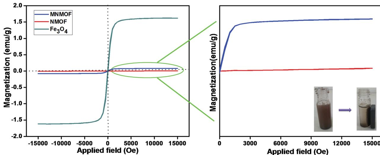
Fig. 2 Hysteresis loops of synthesized  $\text{Fe}_3\text{O}_4$  NPs, NMOF and MNMOF. The inset shows digital images for MNMOF before and after magnetic separation achieved using an external magnetic field.
