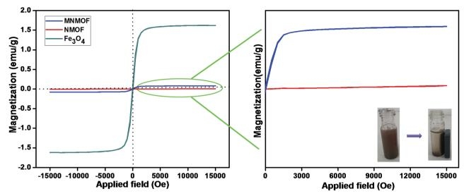
Fig. 2 Hysteresis loops of synthesized  $Fe_3O_4$  NPs, NMOF and MNMOF. The inset shows digital images for MNMOF before and after magnetic separation achieved using an external magnetic field.
