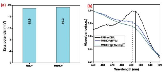
Fig. 7 (a) Zeta-potentials of NMOF and MNMOF, (b) UV-visible spectra of FAM-ssDNA, MNMOF@FAM-ssDNA, and MNMOF@FAM-ssDNA + Hq(II).
