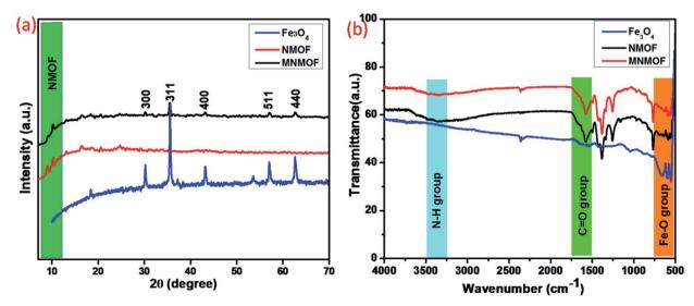
Fig. 1 (a) PXRD patterns of Fe<sub>x</sub>O<sub>4</sub> NPs, NMOF and MNMOF, (b) FT-IR spectra of Fe<sub>x</sub>O<sub>4</sub> NPs, NMOF and MNMOF.
