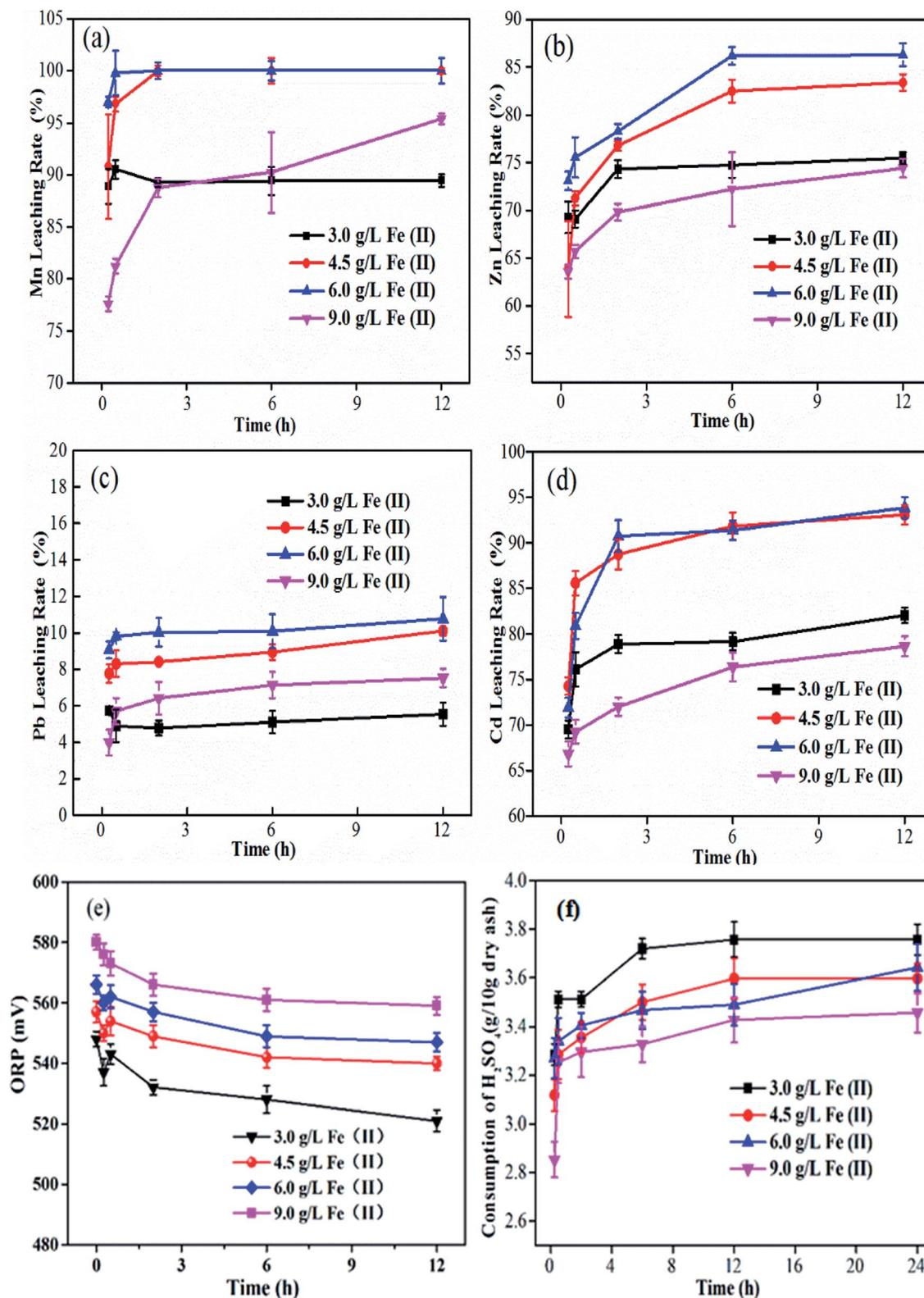
Fig. 1 Variations in bioleaching rates of Mn (a), Zn (b), Pb (c), Cd (d); the redox potential (e) and the total H<sub>2</sub>SO<sub>4</sub> consumption (f) over time with different Fe(II) concentrations.
