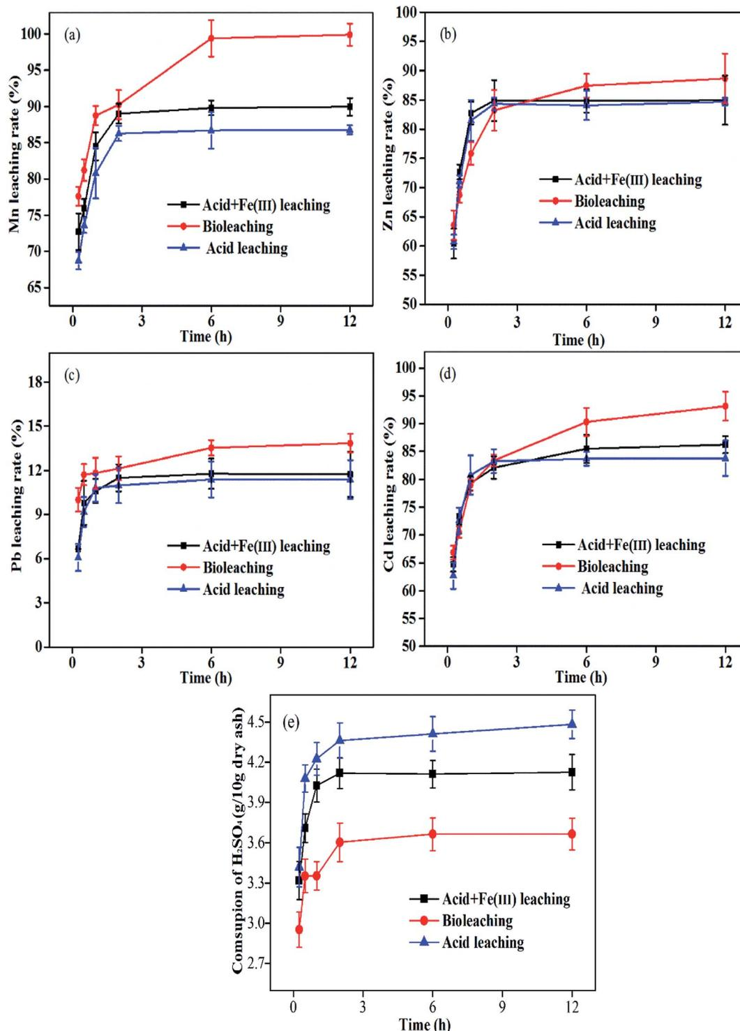
Fig. 4 Comparison of acid leaching, 'Acid + Fe(III)' leaching and bioleaching in stirred tank reactors: leaching rates of Mn (a), Zn (b), Pb (c) and Cd (d), and the total  $\text{H}_2\text{SO}_4$  consumption (e).
