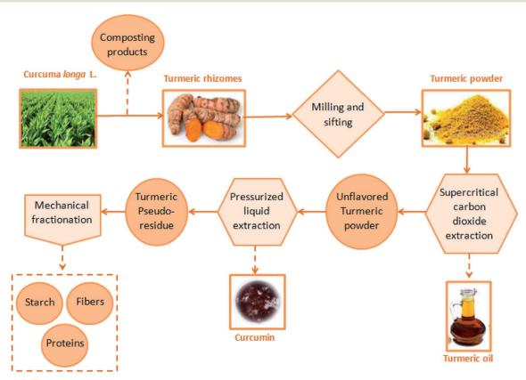
Fig. 2 Turmeric's biorefinery from clean emerging technologies.<sup>7,14</sup>
