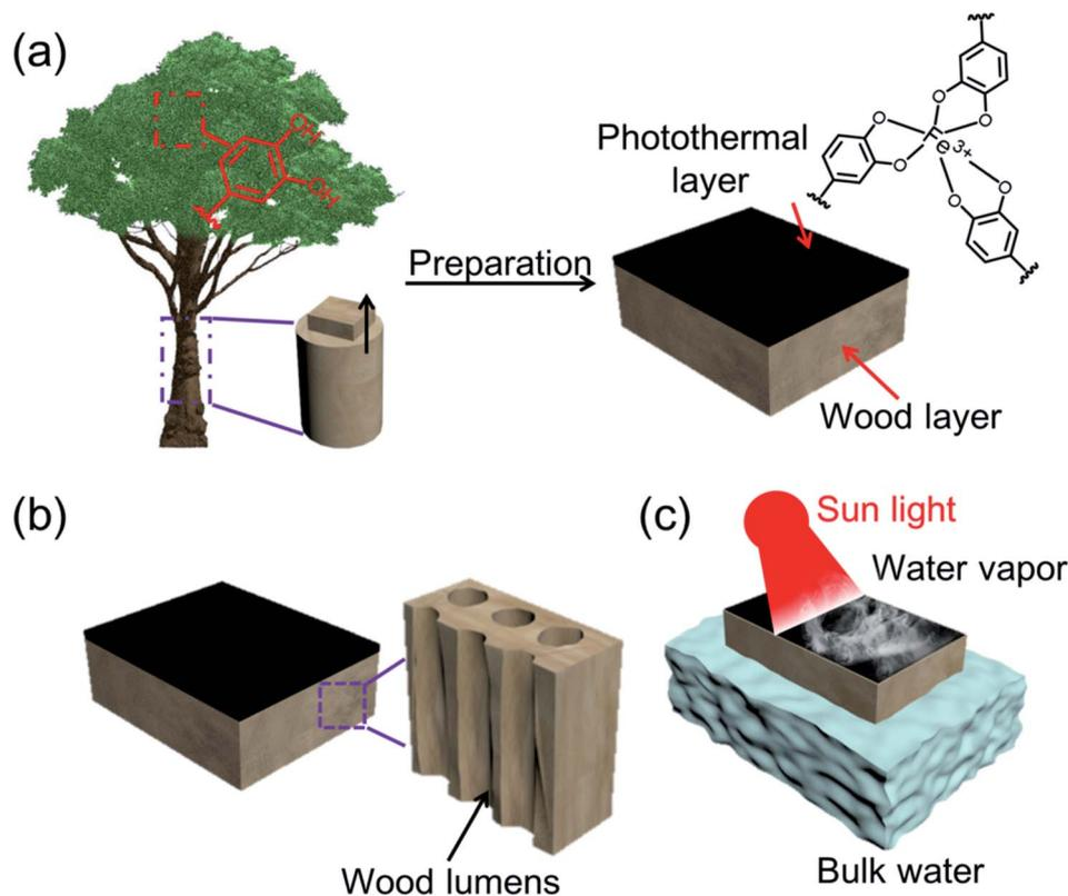
Fig. 1 Schematic illustration of (a) preparation of W-SSGD; (b) magnified structure of wood; (c) solar desalination of sea water.
