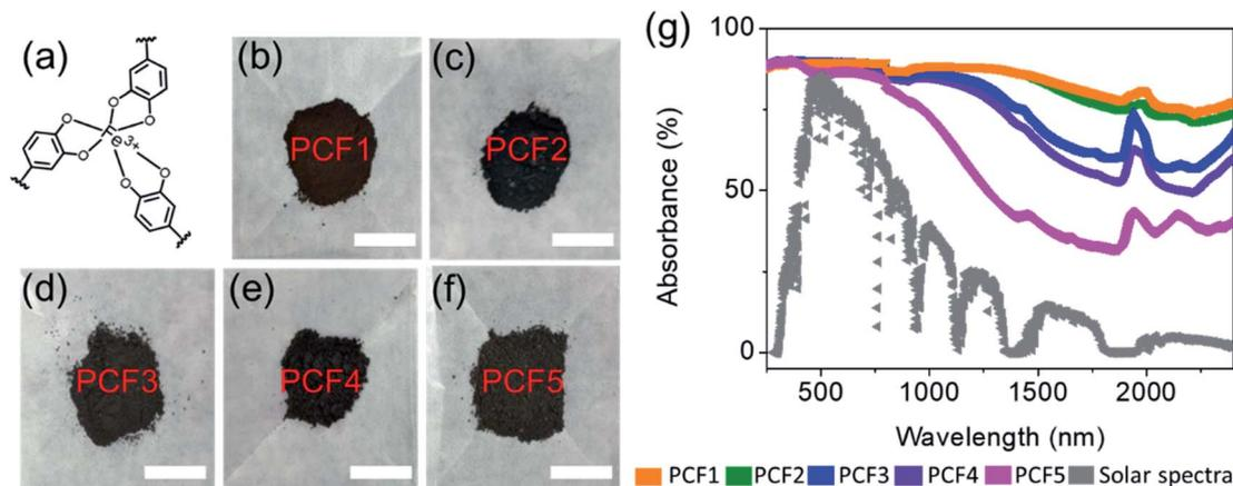
Fig. 2 (a) Possible structure of coordination complexes PCF-*n* (*n* = 1–5); (b–f) images of PCF-*n* (*n* = 1–5) powders, scale bar = 1 cm; (g) absorbance spectra of PCF-*n* (*n* = 1–5) and solar irradiation spectrum.
