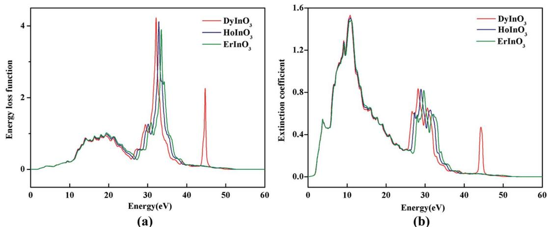
Fig. 7 The electron energy loss spectrum (a) and molar extinction coefficient (b) of hexagonal DyInO<sub>3</sub>, HoInO<sub>3</sub> and ErInO<sub>3</sub>.
