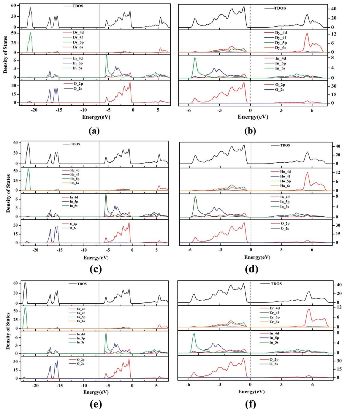
Fig. 3 The total and partial density of states of hexagonal  $\text{DyInO}_3$  (a),  $\text{HoInO}_3$  (c) and  $\text{ErInO}_3$  (e) in the energy range from  $-27$  to  $7$  eV and the enlarged map of  $\text{DyInO}_3$  (b),  $\text{HoInO}_3$  (d) and  $\text{ErInO}_3$  (f) in energy range from  $-7$  to  $7$  eV.
