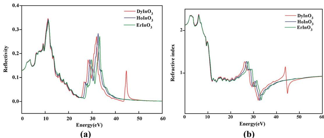
Fig. 6 The reflectivity (a) and refractive index (b) of hexagonal DyInO<sub>3</sub>, HoInO<sub>3</sub> and ErInO<sub>3</sub>.
