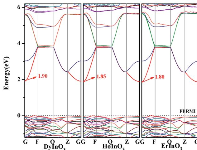
Fig. 2 Band structure of hexagonal  $\text{DyInO}_3$ ,  $\text{HoInO}_3$  and  $\text{ErInO}_3$  along the high symmetry direction. The Fermi level is positioned at zero energy and marked with dotted line.
