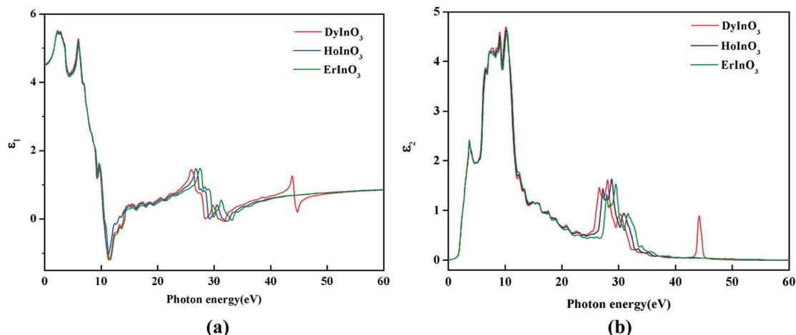
Fig. 4 The real part (a) and the imaginary part (b) of the static dielectric function of hexagonal DyInO<sub>3</sub>, HoInO<sub>3</sub> and ErInO<sub>3</sub>.
