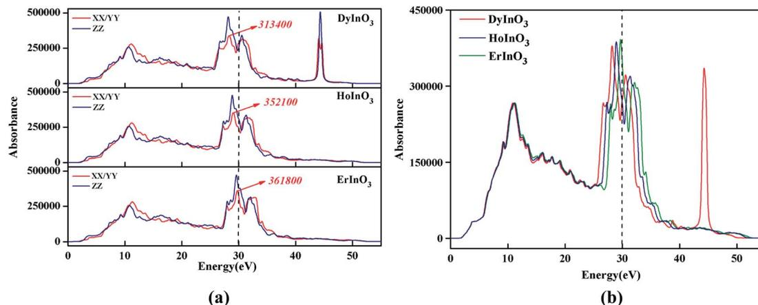
Fig. 5 Absorption spectra of hexagonal DyInO<sub>3</sub>, HoInO<sub>3</sub> and ErInO<sub>3</sub> along different directions respectively (a) and their comparison of total absorption spectra (b) in energy range from 0 to 60 eV.
