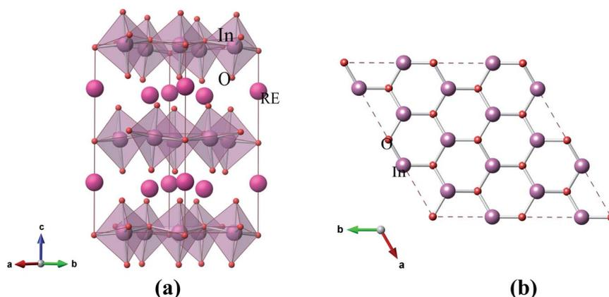
Fig. 1 (a) Optimized structure of hexagonal  $\text{RInO}_3$  ( $\text{R} = \text{Dy, Er, Ho}$ ). (b) Quadrilateral arrangement of a  $2 \times 2 \times 1$  super-cell of optimized hexagonal  $\text{RInO}_3$  along  $c$ -axis.
