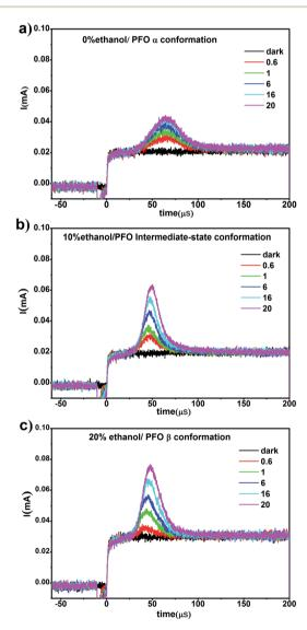
Fig. 7 The photo-CELIV transient current curves of the films obtained from PFO toluene ( $10 \text{ mg mL}^{-1}$ )/ethanol mixed solutions with different ethanol percentages. (a) with 0% ethanol; (b) with 10% ethanol; (c) with 20% ethanol.
