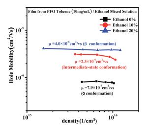
Fig. 8 The hole mobility and charge density curves of the films obtained from PFO toluene (10 mg mL<sup>-1</sup>)/ethanol mixed solutions with different ethanol ratios of 0%, 10% and 20%, respectively.
