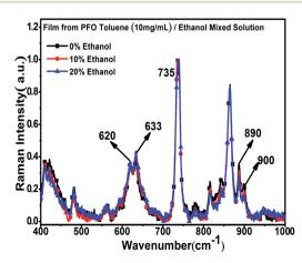
Fig. 3 Raman spectra of the PFO films in the low wave number region with different ethanol contents. All concentrations of the PFO precursor toluene solutions were 10 mg mL<sup>-1</sup>.
