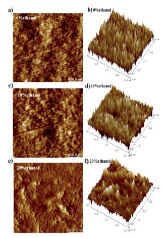
Fig. 6 AFM images of PFO films prepared from PFO toluene (10 mg mL<sup>-1</sup>)/ethanol mixed solutions with different percentages of ethanol. (a) and (b) with 0% ethanol; (c) and (d) with 10% ethanol; (e) and (f) with 20% ethanol.
