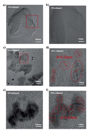
Fig. 5 TEM (left) and HR-TEM (right) images of PFO films prepared from PFO toluene (10 mg mL<sup>-1</sup>)/ethanol mixed solutions with different percentages of ethanol. (a) and (b) with 0% ethanol; (c) and (d) with 10% ethanol; (e) and (f) with 20% ethanol
