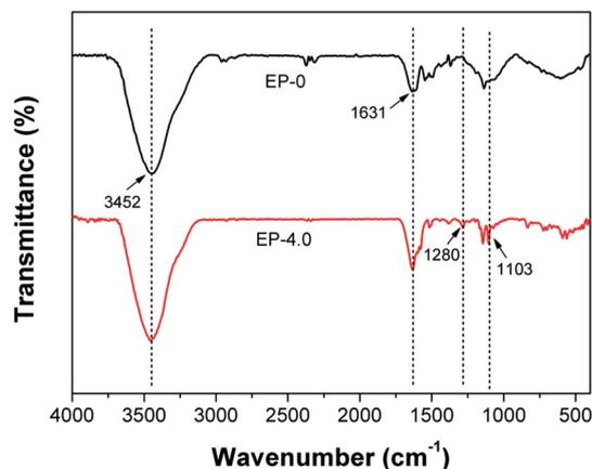
Fig. 10 FT-IR spectra of char residues after CCT.
