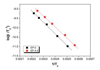
Fig. 6 Plot of  $\ln(\beta/T_{\rm p}^{\,2})$  versus  $1/T_{\rm p}$  of EP-0 and EP-4.0 according to Kissinger's method.
