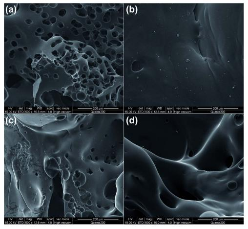
Fig. 9 SEM photographs of external ((a) EP-0, (b) EP-4.0) and internal char layers ((c) EP-0, (d) EP-4.0) after CCT.
