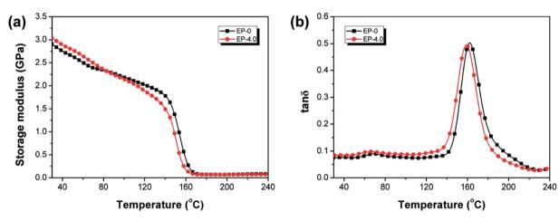
Fig. 13 (a) Storage modulus and (b)  $\tan \delta$  curves of EP-0 and EP-4.0.
