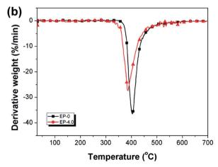
Fig. 11 (a) TGA and (b) DTG curves of EP-0 and EP-4.0 under N<sub>2</sub> conditions.
