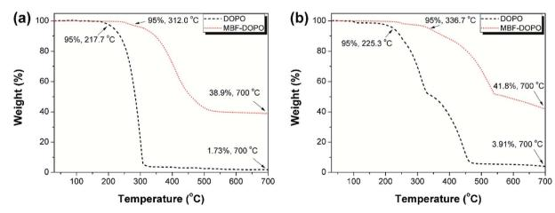
Fig. 4 TGA curves of MBF-DOPO and DOPO under a (a) N<sub>2</sub> and (b) air atmosphere.
