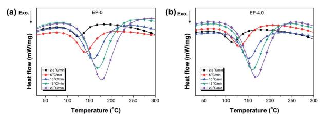
Fig. 5 DSC thermograms of (a) EP-0 and (b) EP-4.0 cured at varying heating rates.
