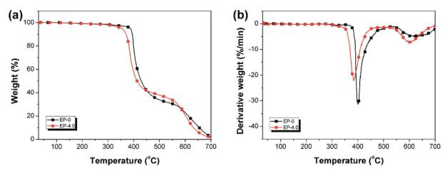
Fig. 12 (a) TGA and (b) DTG curves of EP-0 and EP-4.0 under air conditions.
