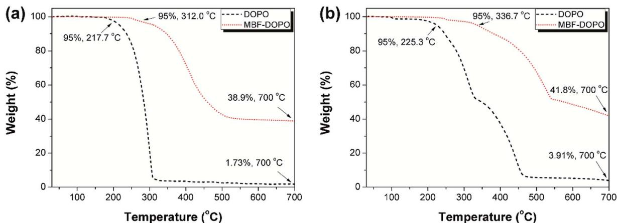
Fig. 4 TGA curves of MBF-DOPO and DOPO under a (a) N<sub>2</sub> and (b) air atmosphere.
