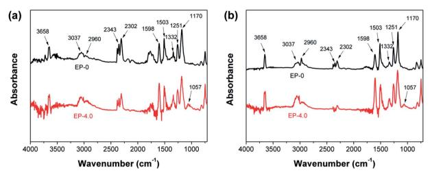
Fig. 8 FTIR spectra of the pyrolysis products of EP-0 and EP-4.0 at (a) the initial and (b) maximum degradation temperatures.
