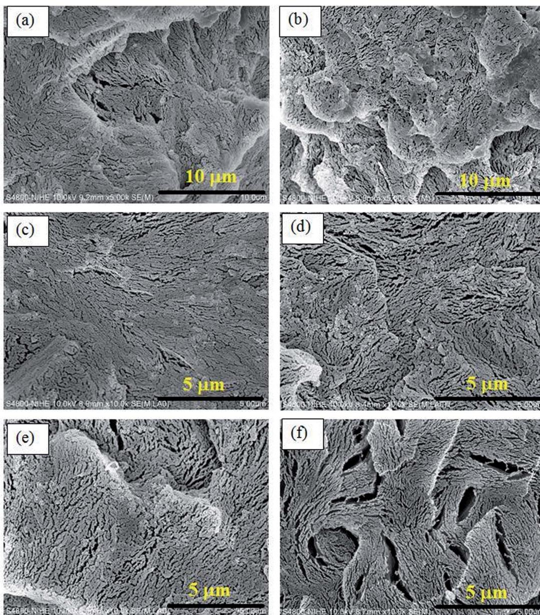
Fig. 8 FESEM images of impact-fractured surfaces of POM and the nanocomposites at magnification of 5000 $\times$  and 10 000 $\times$ : (a) POM, (b) OPELA, (c) 1PELA, (d) 2PELA, (e) 3PELA, and (f) 5PELA.
