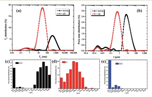
Fig. 9 Results of NMR: comparisons of (a) relaxation time,  $T_2$  distribution and (b) pore size distribution after healing with brine and oil. Pore throat distribution of healed salt with (c) brine (A2-50-1) and (d) oil (A2-50-2). (e) Blank (A2-50-3) without brine and oil is for comparison.
