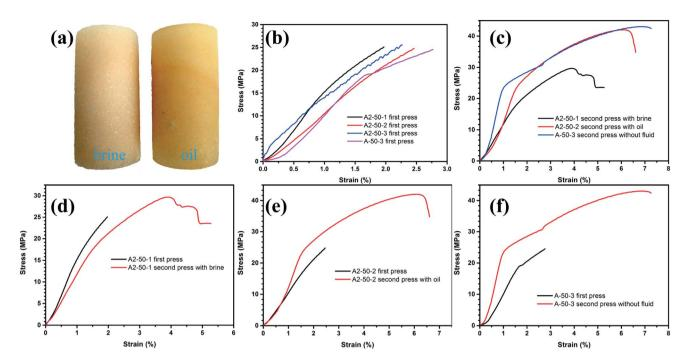
Fig. 4 (a) Photograph of cylindrical salt samples after immersed in saturated brine and oil for 7 days. Stress-strain curves of (b) first test (initial damage), (c) second test, and (d-f) comparisons between both tests.
