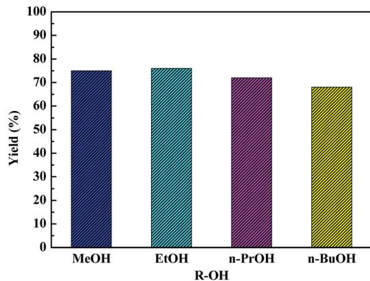
Fig. 10 The catalytic effectiveness of HPW<sub>4</sub>Mo<sub>10</sub>O<sub>x</sub>-Cys for the selective dehydration of glucose and further etherification with various aliphatic alcohols. Reaction conditions: glucose = 100 mg, catalyst 20 mg, time = 20 min.
