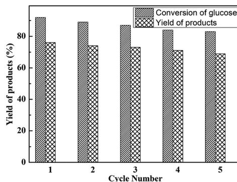
Fig. 11 Reusability study of HPW<sub>4</sub>Mo<sub>10</sub>O<sub>x</sub>-Cys catalyst for glucose dehydration and yields of products. Other reaction condition: glucose = 100 mg, catalyst = 20 mg, at 170 °C for 20 min.
