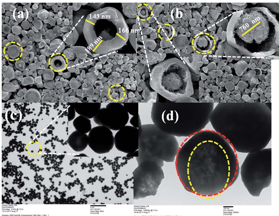
Fig. 1 Representative SEM and TEM images of monodispersed hollow core-shell particles of as-synthesized  $\text{HPW}_4\text{Mo}_{10}\text{O}_x$  materials: (a) and (b) SEM images, scale bar 1  $\mu\text{m}$ ; (c) and (d) TEM images, scale bar 4  $\mu\text{m}$  and 100 nm respectively.
