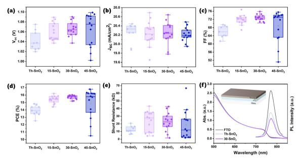
Fig. 4 (a-e) Boxplots of device properties (V<sub>OC</sub>, J<sub>SC</sub>, FF, PCE, and estimated shunt resistance, respectively). (f) UV-vis and PL spectra of perovskite coated on FTO, Th-SnO<sub>2</sub>, and 30-SnO<sub>2</sub>. Inset diagram shows the tested device architecture. Colour scheme is the same as that for Fig. 1b.
