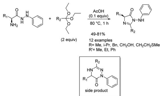
**Scheme 10** Kacem and Hassine's solvent-free synthesis of imidazolones.
