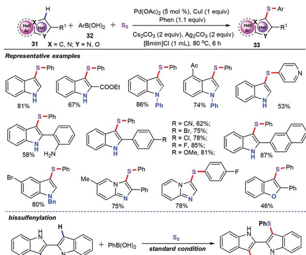
**Scheme 13** Palladium-catalyzed oxidative sulfenylation of electron-rich heteroarenes.
