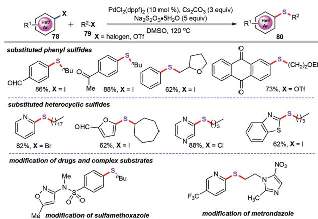
**Scheme 30** Palladium-catalyzed cross-coupling access to diverse aromatic sulfides.
