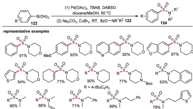
**Scheme 47** Pd/Cu co-catalyzed three-component cascade sulfonylation reaction.
