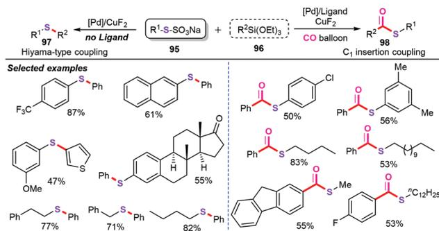
**Scheme 36** Palladium-catalyzed ligand-controlled cross-coupling involving an organosilicon reagent.
