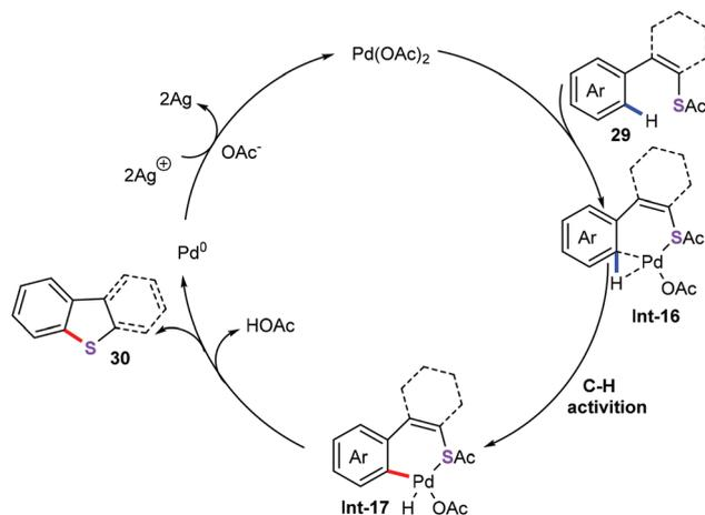
**Scheme 12** Proposed mechanism for the palladium-catalyzed C–S cyclization.
