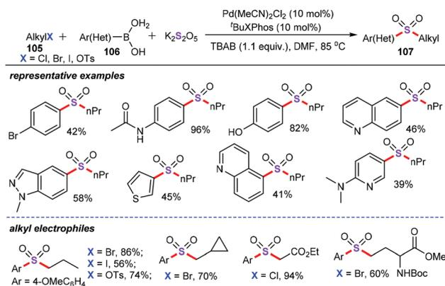
**Scheme 39** Palladium-catalyzed three-component cascade sulfonylation reaction.
