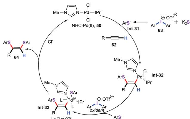
**Scheme 26** Plausible mechanism for palladium-catalyzed three-component cascade bithiolation.
