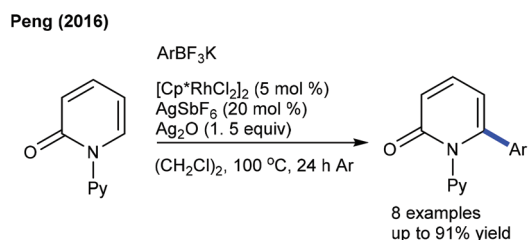
Scheme 7 Arylation of pyridones using aryl trifluoroborates.
