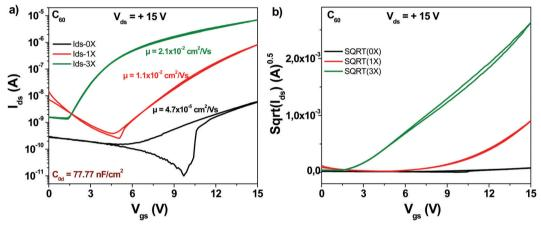
Fig. 5 (a) Comparison of OFET devices with three different grades of fullerene ( $C_{60}$ ) semiconductor purity: unpurified ( $0 \times$  in graph legend), one time purified ( $1 \times$  in graph legend) and three times purified respectively ( $3 \times$  in graph legend); (b) the sqrt( $I_{ds}$ ) vs.  $V_{as}$  of the three purity grades presented in panel (a).
