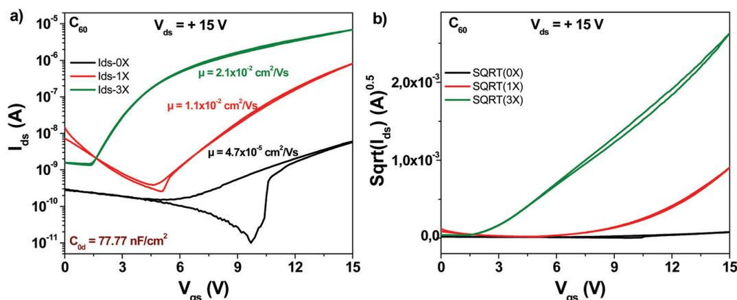
Fig. 5 (a) Comparison of OFET devices with three different grades of fullerene (C<sub>60</sub>) semiconductor purity: unpurified (0x in graph legend), one time purified (1x in graph legend) and three times purified respectively (3x in graph legend); (b) the  $\sqrt{I_{ds}}$  vs.  $V_{gs}$  of the three purity grades presented in panel (a).
