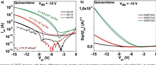
Fig. 9 (a) Comparison of OFET devices with three different purity grades of quinacridone semiconductor: unpurified  $(0 \times \text{in graph legend})$ , one time purified (1× in graph legend) and three times purified, respectively (3× in graph legend); (b) the  $sqrt(I_{ds})$  vs.  $V_{qs}$  of the three purity grades presented in panel (a).
