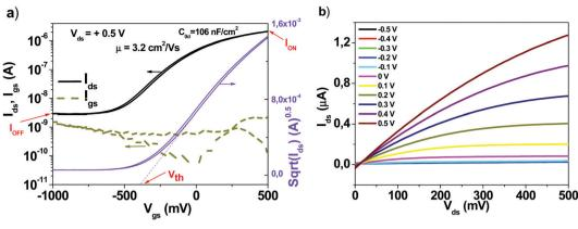
Fig. 3 (a) Transfer and (b) output characteristics of an organic field effect transistor which was part of the same batch as the one presented in ref. 60, as Fig. 4(c and d). Adapted with permission from ref. 60, G. Schwabegger, et al., High Mobility, Low Voltage Operating C<sub>60</sub> based n-type Organic Field Effect Transistors, Synth. Met., 2011, 161, 2058-2062.
