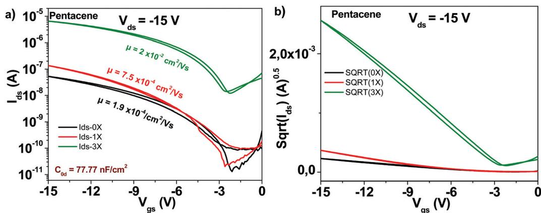
**Fig. 6** (a) Comparison of OFET devices with three different purity grades of pentacene semiconductor: unpurified (0x in graph legend), one time purified (1x in graph legend) and three times purified respectively (3x in graph legend); (b) the  $\sqrt{I_{ds}}$  vs.  $V_{gs}$  of the three purity grades presented in panel (a).
