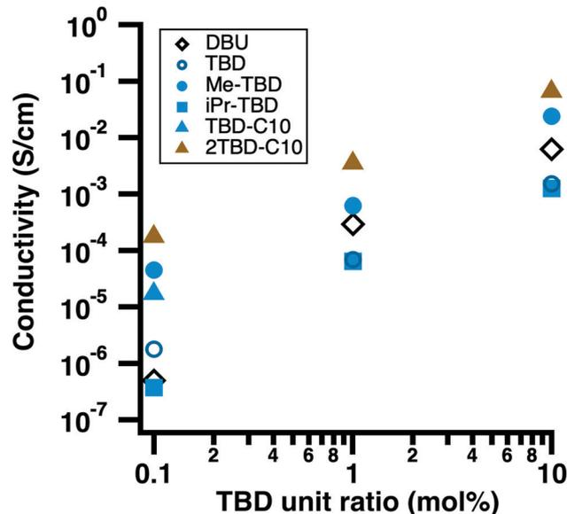
Fig. 2 Electrical conductivities of films of  $\text{PC}_{61}\text{BM}$  doped with **TBD**-derivatives and DBU as a function of the molar ratio. **TBD-C10** has a data point only at 0.1 mol% because films could not be cast at higher molar ratios.
