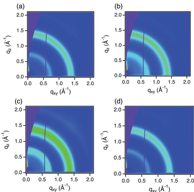
Fig. 3 2-Dimensional GIWAXS images of (a) pristine PC<sub>61</sub>BM, (b) PC<sub>61</sub>BM with 10 mol% **2TBD-C10**, (c) PC<sub>61</sub>BM with 10 mol% **Me-TBD**, and (d) PC<sub>61</sub>BM with 10 mol% **iPr-TBD**.
